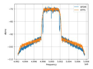
Fig. 7: Power spectral density of OFDM and OTFS.
