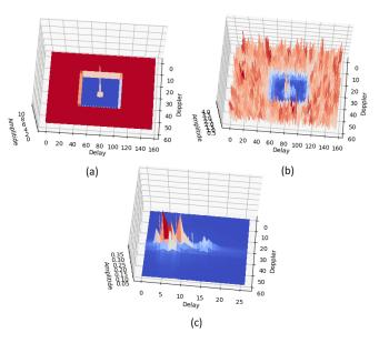
Fig. 4: (a) QPSK data in the OTFS resource grid. (b) The grid at the receiver and after applying the channel. (c) The channel response in DD domain
