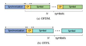
Fig. 2: Time slot structure for transmission with OFDM and OTFS.
