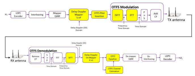
Fig. 1: OTFS transceiver architecture.
