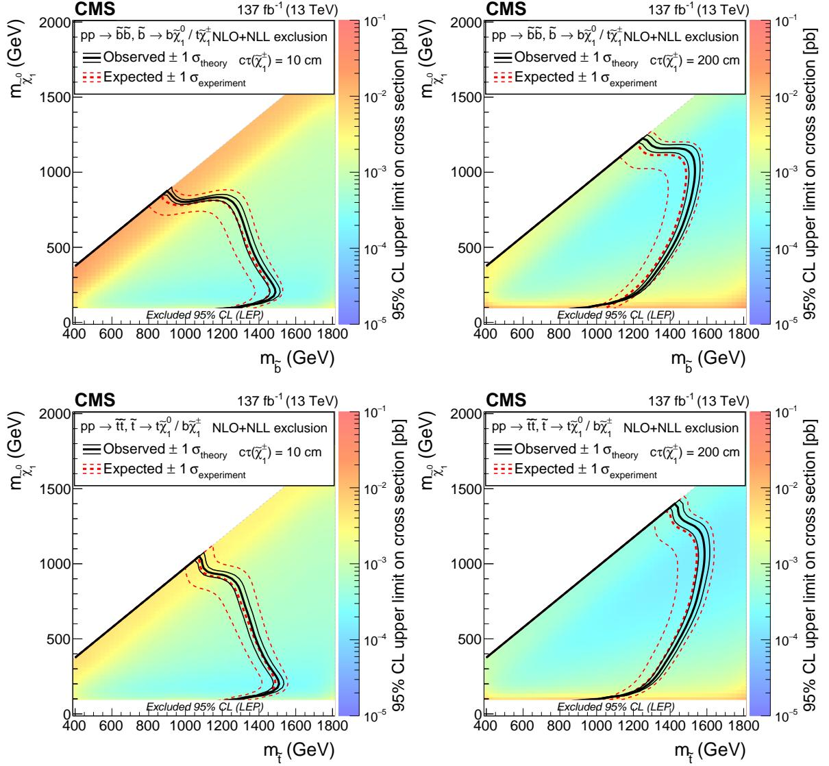
Figure 10: Observed 95% CL upper limits on the signal cross sections (colored area) versus the bottom or top squark and neutralino mass for the T6tbLL (upper) and T6btLL (lower) model for a chargino proper decay length  $c\tau$  of 10 (left column) or 200 (right column) cm. Also shown are black (red) contours corresponding to the observed (expected) lower limits, including their uncertainties, on the squark and neutralino masses.
