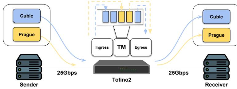
**Fig. 8** Evaluation setup. Cubic and Prague flows coexist in the same scenario, sharing the programmable switch bandwidth.
