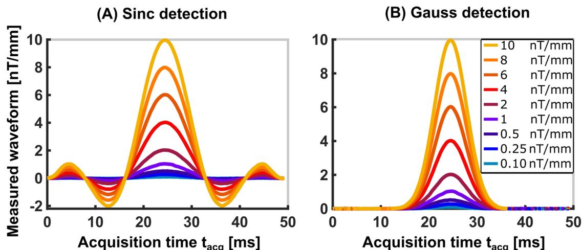
**Supplementary Figure 1)** Measured gradient trajectories for a Sinc- and Gauss-shaped stimulus of 50 ms duration at  $t \cdot BW = 6$ . The validation was performed on a spherical phantom (diameter 17.5 cm) of demineralized water doped with 1.25 g/L  $\text{NiSO}_4$  in a slice with 50 mm offcenter distance and 2 mm slice thickness. The gradient amplitude was varied between 0.1 and 10 nT/mm which corresponds to a peak amplitude of 1 to 100 nT in a slice at 10 mm offcenter distance.
