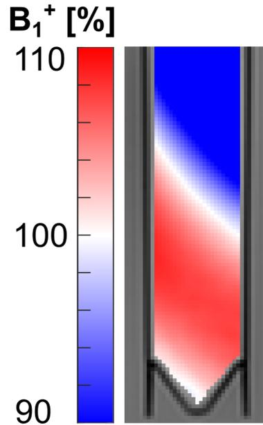
**Supplementary Figure 3)** Corrected transmission field amplitude in the BSA phantom. Due to the correction with a factor of 1.23 determined from preliminary experiments and the installation of the small sample in a large water phantom containing NaCl, the transmitted SL field deviates only slightly from its nominal value.
