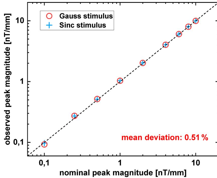
Supplementary Figure 2) Control of the peak magnitudes of the calibrated waveforms. The observed values were compared with the nominal values. An average deviation of 0.51 % was determined.
