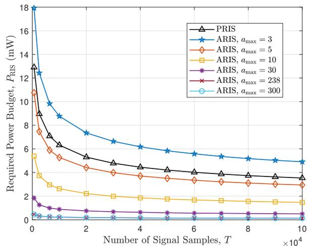
Fig. 3. The required power budget to realize a target detection probability of 0.9 for different  $T$ 's under the case with negligible interferers.
