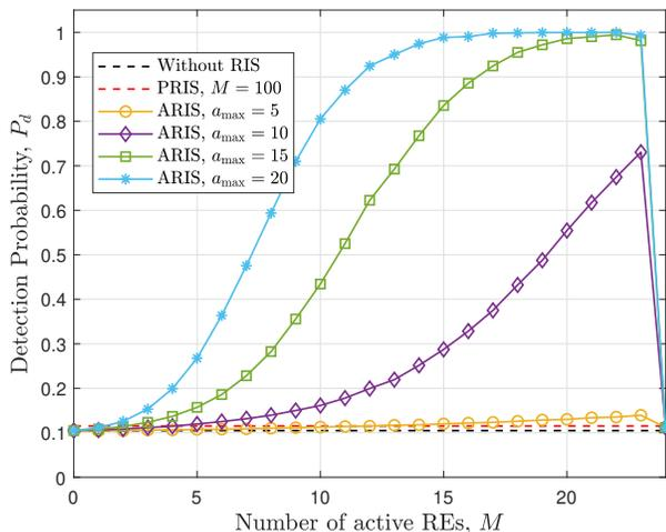
Fig. 2. The performance gains of the active RIS and passive RIS on the detection probability.
