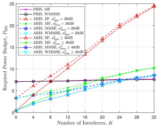
Fig. 7. The required power budget to realize a target detection probability of  $P_d = 0.9$  for different numbers of the interferers.
