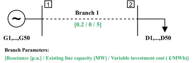
Fig. 4. Topology of the 2-node transmission network.
