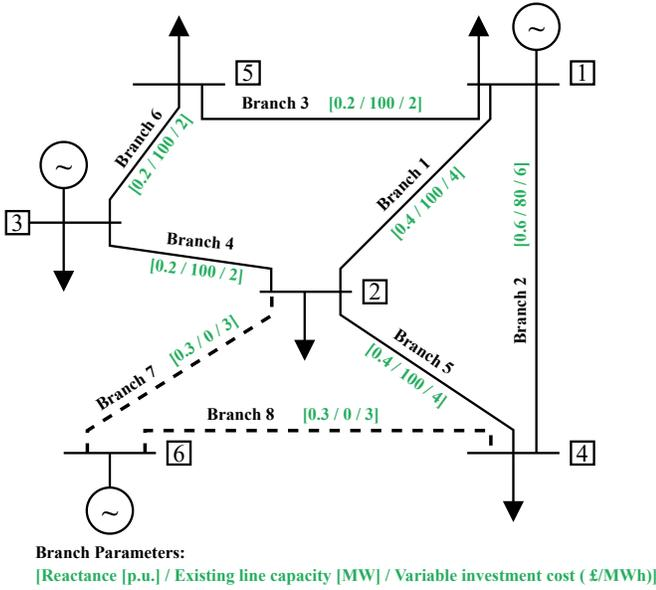
Fig. 6. Topology of the Garver's 6-node transmission network.
