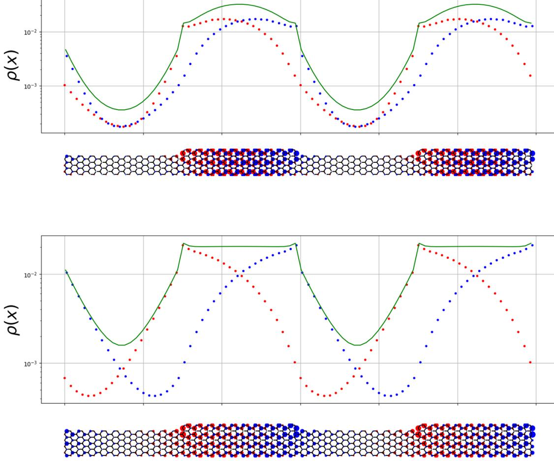
Figure 12. Lowest energy state densities of a 7/9-junction (top) and a 9/11-junction (bottom) with  $(m_N, m_{N+2}) = (10, 10)$  and aligned at the bottom rather than the center. According to Ref. [8] the 9/11-junction features a change in the topology of the respective armchairs (see table I). Both cases are Kilimanjaro-localised since the 9- and 11-armchair sides, respectively, exhibit long range correlations.
