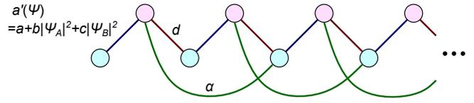
FIG. 1. **Schematics of the long-range nonlinear SSH model.** The model has two sublattices (red and blue circles) and staggered nearest hopping. The strength of the intercell nearest-neighbor hopping depends on the state variables. We also introduce long-range hoppings (green curves) to investigate the effect of higher winding numbers.
