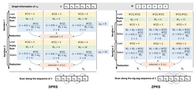
Figure 3: The comparison of DPRS and ZPRS on sampling a neighbor of  $v_0$  in Figure 1a using three threads. DPRS scans W once, but the number of collective operations depends on the number of iterations. ZPRS performs two collective operations only, but scans W twice. Logically, DPRS scans along the sequence of S, whereas ZPRS scans in a zig-zag order of S.
