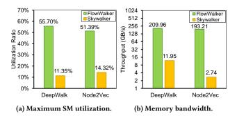
Figure 11: Comparison of GPU resource utilization on LJ.
