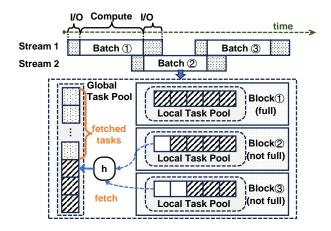
Figure 5: Queries are grouped into batches which execute alternatively in two CUDA streams. h refers to the head pointer of the global task pool. Thread blocks fetch tasks in a preemptive way if they have empty slots.
