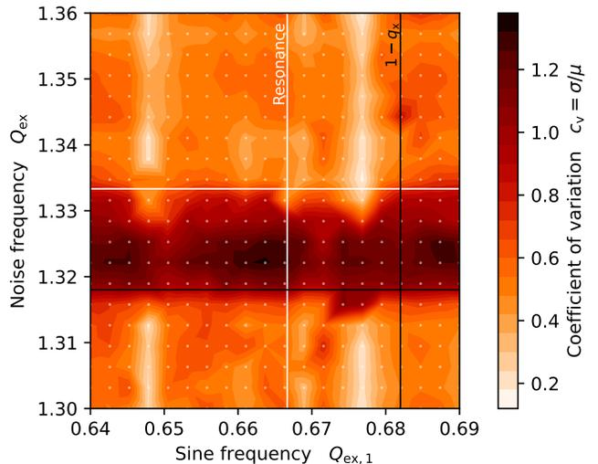
FIG. 7. Measured spill quality as a function of sine and noise frequency for an excitation with Noise++. For the scan, the noise bandwidth  $\Delta Q_{\text{ex}} = 0.01$  and frequency of the second sine  $Q_{\text{ex},2} = 1.6715$  are kept constant.
