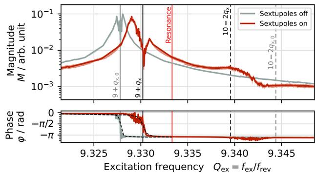
FIG. 2. Measured response to a sinusoidal excitation (BTF measurement) of an  $^{197}\text{Au}^{65+}$  beam at 800 MeV/nucleon. Vertical lines indicate the location of the betatron sidebands and resonance.
