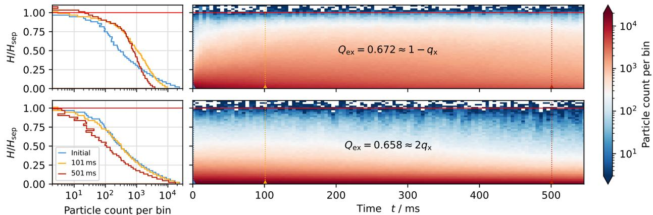
FIG. 6. Particle distributions before and during excitation near the first (top) and second order sideband (bottom) obtained from a simulation of  $10^5$  particles. The band-limited noise excitation signals correspond to figures 3 and 5 ( $\Delta Q_{\text{ex}} = 0.008$ ). The location of the separatrix at  $H = H_{\text{sep}}$  is indicated by the solid red line.
