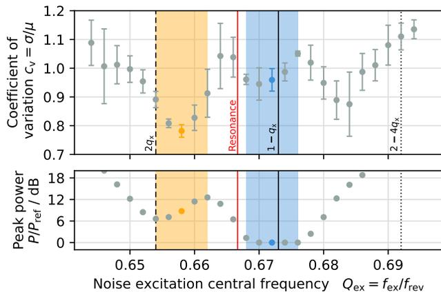
FIG. 5. Spill quality (top) and excitation power (bottom) as function of excitation frequency for a band-limited noise signal ( $\Delta Q_{\text{ex}} = 0.008$ ) as obtained from simulations. The quality is calculated for  $\Delta t_{\text{count}} = 100 \mu\text{s}$  and  $\Delta t_{\text{eval}} = 100 \text{ms}$ . Vertical lines mark the resonance and nearby betatron sidebands, and the two excitation bands from figure 3 are indicated.
