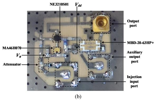
Fig. 2. (a) Schematic of the individual  $i$ -th VCO of the array, where  $V_{dd}$  and  $\eta_i$  are the drain and tuning voltages, respectively. The variables  $L$  and  $W$  represent the length and the width of each line in  $mm$ . (b) Photograph of the individual VCO.
