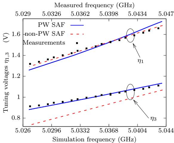
Fig. 11. Injected array. Variation of the tuning voltages  $\eta_{1,3}$  versus the synchronization frequency  $f_s$ . The constant phase shift has been fixed to  $\Delta\varphi = 7\pi/6$  rad and the input generator phase  $\theta_s$  has been swept in the range  $[0, 2\pi]$  rad.
