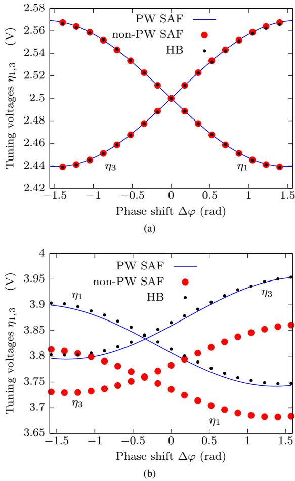
Fig. 6. Array of  $N = 3$  Van der Pol-type oscillators. Simulation of the evolution of  $\eta_{1,3}$  along the stable range of constant phase-shift solutions. (a) Identical oscillators. The tuning voltages vary symmetrically and the PW SAF with  $p = 33$  points, the non-PW SAF and the circuit-level HB techniques provide similar results. (b) Non-identical oscillators. The symmetry of the previous case is broken, and the non-PW SAF technique presents discrepancies with HB and PW SAF techniques.
