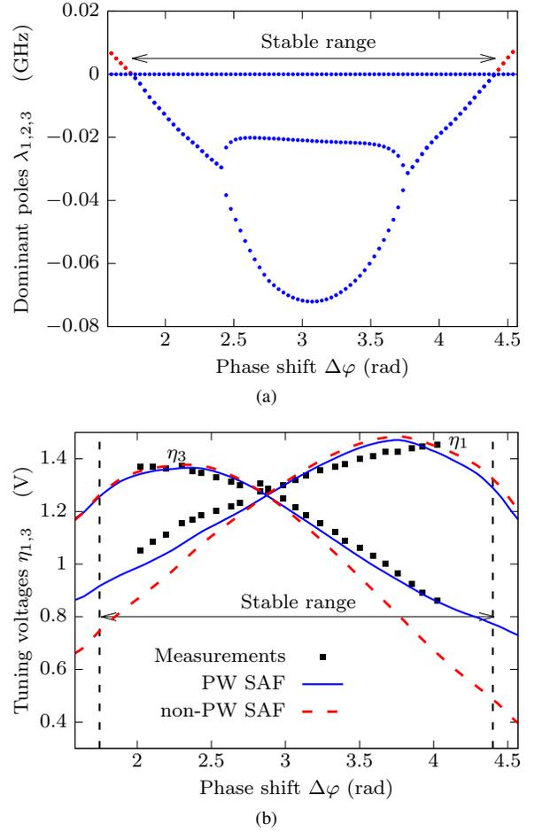
Fig. 8. Free-running array. (a) Evolution of the dominant poles  $\lambda_{1,2,3}$  with the constant phase shift  $\Delta\varphi$ , determining the stable range. (b) Variation of the tuning voltages  $\eta_{1,3}$  versus  $\Delta\varphi$ .
