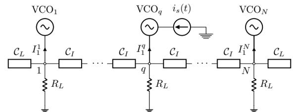
Fig. 4. Schematic of the coupled oscillator array. The output port of each oscillator element is loaded with a resistor  $R_L = 50 \Omega$  and coupled to the neighbor elements through a linear network.
