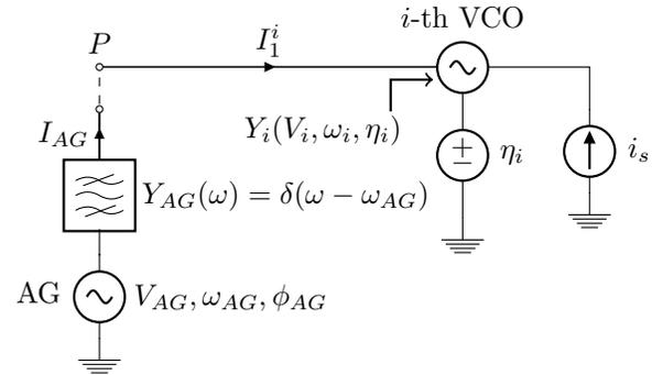
Fig. 1. Procedure to extract the model of the individual  $i$ -th VCO. An auxiliary generator (AG) is connected to the output node  $P$  to calculate the first-harmonic input admittance function  $Y_i(V_i, \omega_i, \eta_i)$  and the derivatives  $I_{iG_{\pm 1}}(V_i, \omega_i, \eta_i)$  providing the dependence of the input current  $I_1^i$  on the injection source  $i_s(t)$ .
