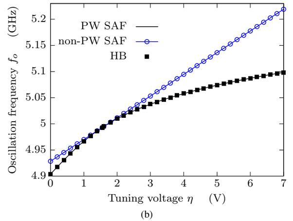
Fig. 3. Evolution of the free-running steady state solution versus the tuning voltage  $\eta$ . Comparison of the results obtained with the non-PW SAF with the PW SAF. The PW SAF agrees with the circuit-level HB simulations at the points  $\eta_i$  of the sampling interval. (a) First harmonic amplitude  $V_o$ . (b) Oscillation frequency  $f_o$ .
