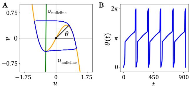
FIG. 4 **From a limit cycle oscillator to a phase oscillator.** A. The depicted limit cycle is transformed into a phase oscillator by employing the arctangent function to define the phase variable. B. This transformation yields a new variable  $\theta$  that exhibits periodic oscillations, maintaining the original cycle’s two fast and two slow segments. The parameters used here are consistent with those in Fig. 1C.
