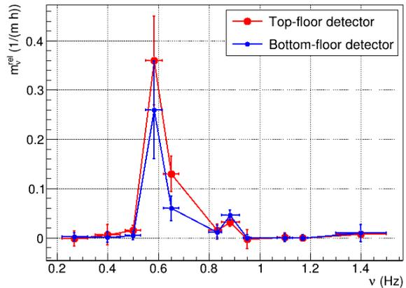
**Fig. 10** Sensitivity of the the low-frequency noise components to changes of the sea activity for two detectors, at the bottom and at the top of a CUORE tower.
