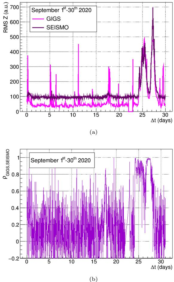
**Fig. 2** Time evolutions of GIGS and SEISMO RMS Z (a) and of their correlation coefficient (b) in September 2020. The spikes of high correlation can be attributed to earthquakes, since they affect all the seismometers.
