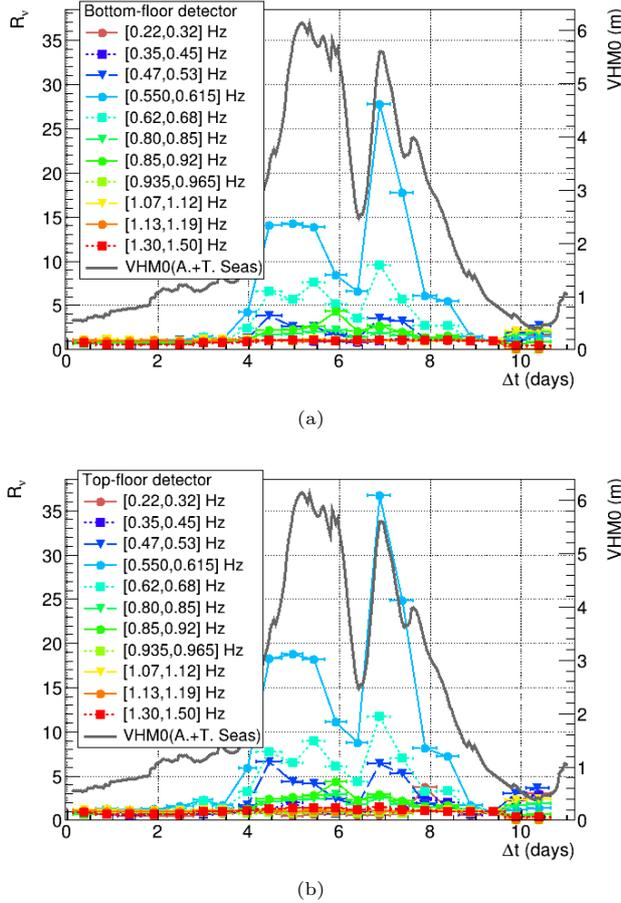
**Fig. 8** Comparison between the time evolutions of the sea waves height and of the noise power ratio  $R_\nu$  for various frequency components of the noise, for two detectors placed at the bottom (a) and at the top (b) floors of a CUORE tower.
