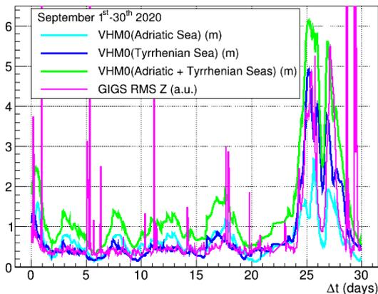
**Fig. 4** Comparison between the time profiles of VHM0 for Adriatic Seas, Tyrrhenian Sea and for their combined contribution, and the time profile of RMS Z of GIGS seismometer (rescaled by a constant factor for a better comparison with VHM0 data), during September 2020.
