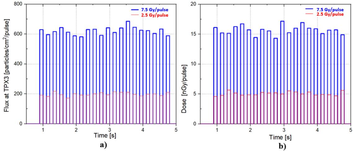
**Figure 3.** Evaluation of scattered radiation field at the TPX3 detector out-of-field position. Measured (a) particle flux and (b) DPP in the TPX3 detector are shown for the same LINAC configurations as in Figure 2. Results are given for 20 pulses (corresponding to 4 s of beam-on irradiation).
