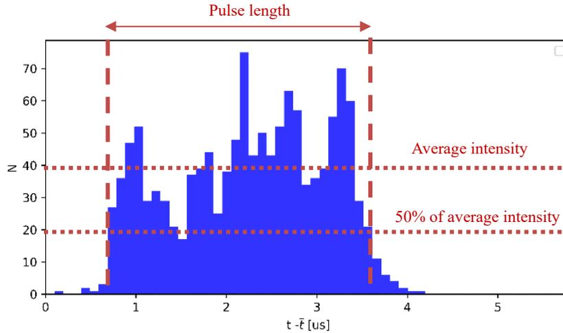
**Figure 6.** The measured particle count for one selected pulse from campaign number 7 as a function of time is shown with the pulse's initiation at  $\bar{t} \sim 4s$ . The measured data were binned into time intervals of 100 ns. The dotted horizontal lines mark average pulse intensity and 50 % of average pulse intensity. Vertical dashed lines indicate the start and the end of a pulse.
