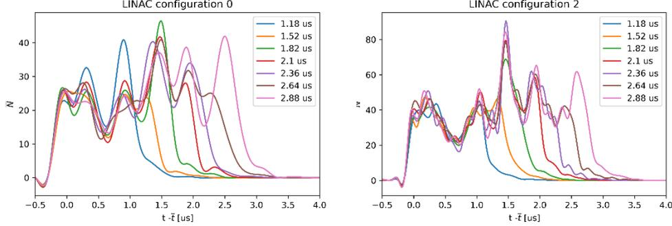
**Figure 8.** Measured temporal pulse nanostructure across various lengths for the two LINAC configurations. The data were binned into 200 ns and 100 ns time intervals for configurations “2” and “0”, respectively, to ensure sufficient data in a bin. The binned data were smoothed for visual purposes,  $\bar{t}$  denotes the start of a pulse as defined in Section 3.4.
