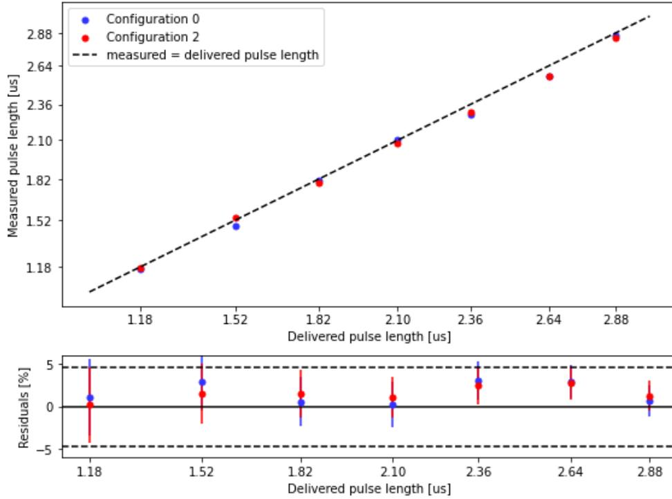
**Figure 7.** Upper panel: Measured pulse lengths as a function of delivered pulse lengths for campaigns 1-7 and 15-21 for LINACS configurations “2” and “0”, respectively. Lower panel: Residuals of average measured pulse lengths are well within the margin of average relative error of delivered pulse lengths, denoted by dashed lines in the Residuals subplot. Error bars represent type A uncertainty for TPX3 pulse length measurements.
