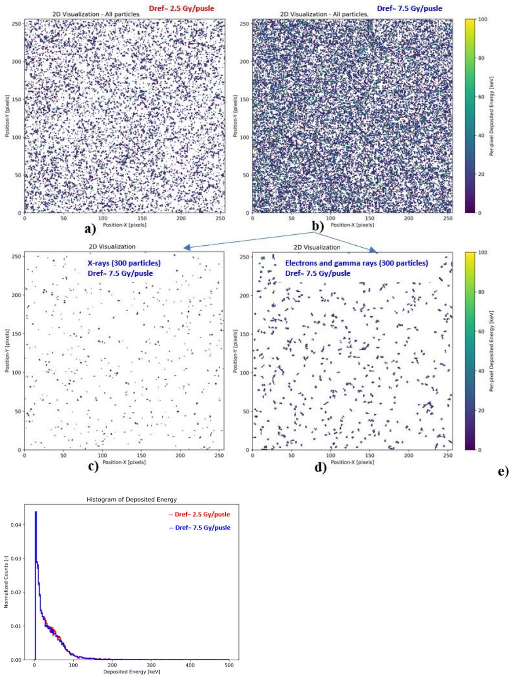
**Figure 2.** a), b) Visualization of the detected secondary radiation particles. Integrated deposited energy maps are shown for all delivered 20 pulses measured. Radiation field decomposition into two classes of particles for data from Figure b): c) low-energy X-rays (below 30 keV) and d) electrons and gamma rays (above 30 keV). e) The normalized histogram of deposited energy spectra of measured single particles from campaigns 14 and 7.
