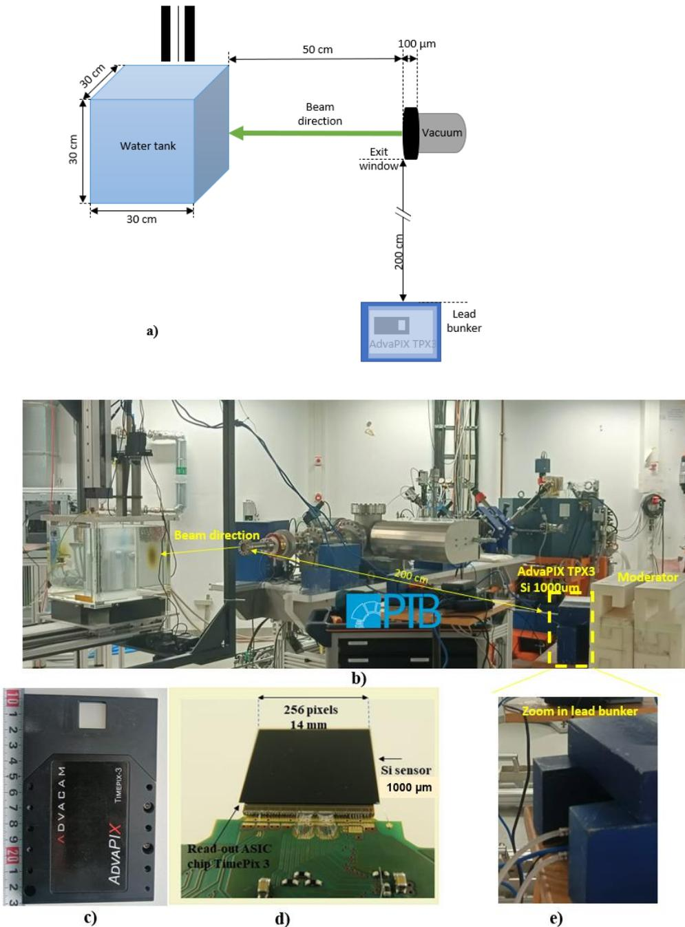
**Figure 1.** a) Schematic representation of the experimental setup b) picture from the experimental room, c) Advapix TPX3 detector, d) its ASIC chip and silicon sensor of 1000  $\mu\text{m}$  thickness, and e) the detector was placed in a lead bunker.
