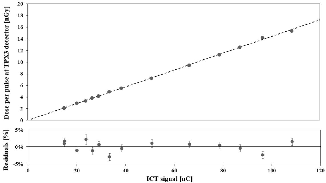
**Figure 4.** DPP measurement with TPX3 detector as a function of the beam delivered monitored by the ICT. The linear regression coefficient of determination is calculated to be  $R^2 \sim 1$ . The lower graph shows the residual from the linear fit. The error bar represents  $k=1$ .
