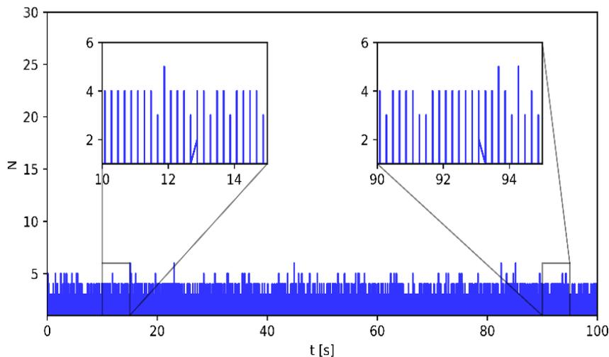
**Figure 5.** *Out-of-field scattered particle count generated by UHDPP electron beams as measured by the TPX3 detector. The zoomed-in windows with 5 s time intervals allow for visualization of individual pulses.*
