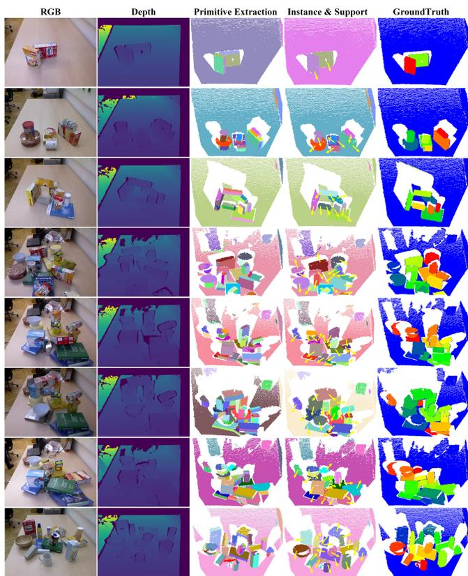
Fig. 12. Experimental results of our algorithm. The first and second columns are RGB and depth images, respectively, from the OSD dataset. The middle column is the initial over segmentation of abstracting the scene to planar primitives. The primitive classification and support relations inference results are presented in the fourth column. The ground truth of the segmentation is shown in the last column.
