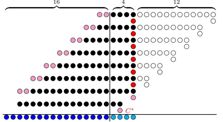
Figure 2. A 16-bit commutative truncated Booth multiplier, with 12 columns of truncation. The six red bits are the additional compensation bits  $s'_i$ . The pink bits represent the typical Booth sign bits  $s_i$ .
