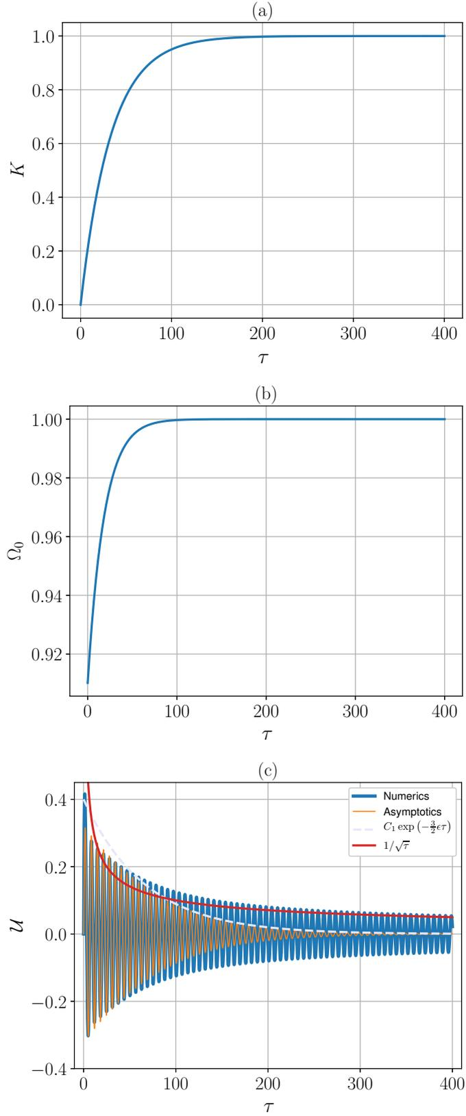
Figure 6: (a) Given time-varying parameter  $K$ , (b) the trapped mode frequency  $\Omega_0$ , (c) the displacement  $\mathcal{U}$  of the discrete sub-system for the case when parameters are taken according Eqs. (7.14), (7.15)
