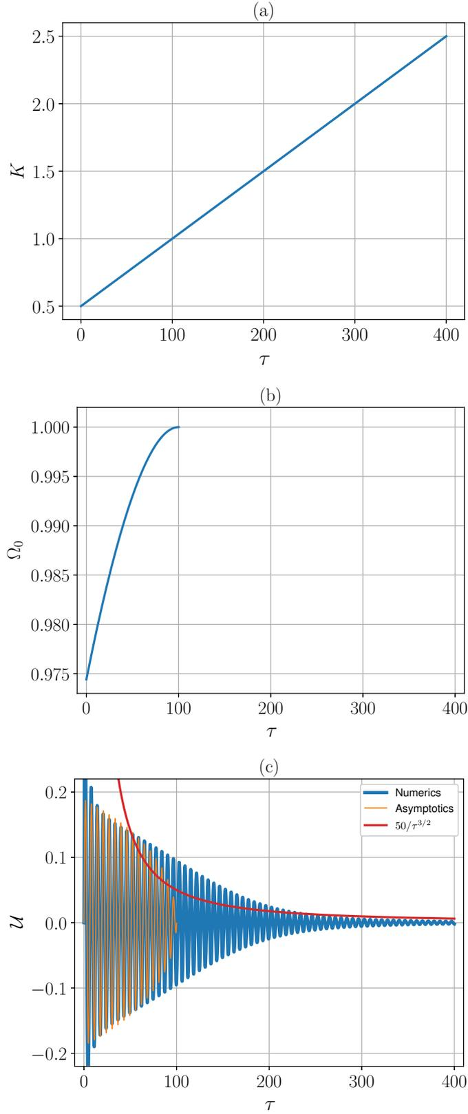
Figure 7: (a) Given time-varying parameter  $K$ , (b) the trapped mode frequency  $\Omega_0$ , (c) the displacement  $\mathcal{U}$  of the discrete sub-system for the case when parameters are taken according Eqs. (7.14), (7.15)
