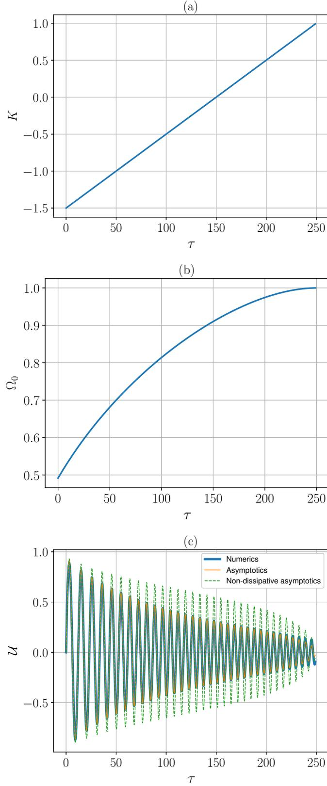
Figure 4: (a) Given time-varying parameter  $K$ , (b) the trapped mode frequency  $\Omega_0$ , and (c) the displacement  $\mathcal{U}$  of the discrete sub-system for the case when parameters are taken according Eq. (7.6), (7.7) wherein  $K_0 = -1.5$ ,  $K_1 = 1.0$
