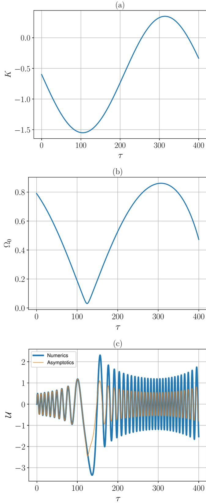
Figure 5: (a) Given time-varying parameter  $K$ , (b) the trapped mode frequency  $\Omega_0$ , (c) the displacement  $\mathcal{U}$  of the discrete sub-system for the case when parameters are taken according Eqs. (7.3), (7.4), (7.13)
