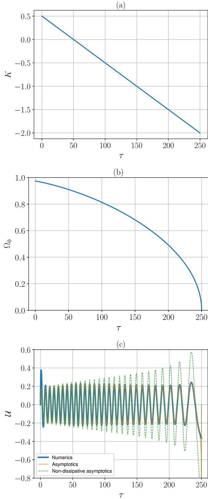
Figure 3: (a) Given time-varying parameter  $K$ , (b) the trapped mode frequency  $\Omega_0$ , and (c) the displacement  $\mathcal{U}$  of the discrete sub-system for the case when parameters are taken according Eq. (7.6), (7.7) wherein  $K_0 = 0.5$ ,  $K_1 = -1.0$
