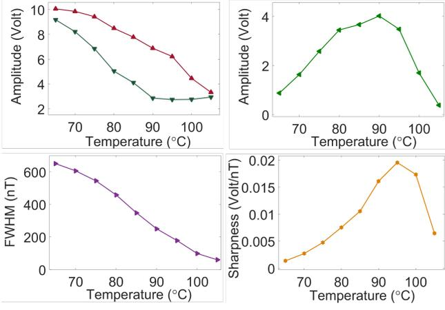
FIG. 3. ZFR parameters versus LWVC temperature, acquired with pump power of  $360 \mu\text{W}$ . C.f. Fig. 2 and Eq. (1). (upper left) photodetector voltage minimum  $a$  (green) and maximum  $b$  (red)  $b$ . (upper right) amplitude  $b - a$ . (lower left) FWHM linewidth  $\Delta B$ . (lower right) sharpness  $s = (b - a)/\Delta B$ , showing an optimum at  $96^\circ\text{C}$ .
