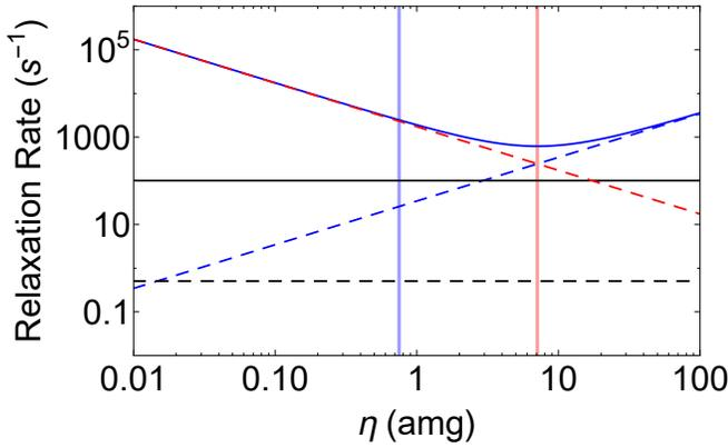
FIG. 5. Collisional relaxation rates as a function of  $N_2$  buffer gas density at  $T = 96^\circ\text{C}$ .  $\Gamma_{\text{wd}}^{\text{LWVC}}$  (dashed red),  $\Gamma_{\text{bg}}$  (dashed blue),  $\Gamma_{\text{sd}}$  (dashed black),  $\Gamma_{\text{se}}$  (continuous black), total  $\Gamma_{\text{dk}}$  (continuous blue). Experimental (optimal) nitrogen density is indicated with a vertical blue (red) line at 0.75 amg (7.1 amg).
