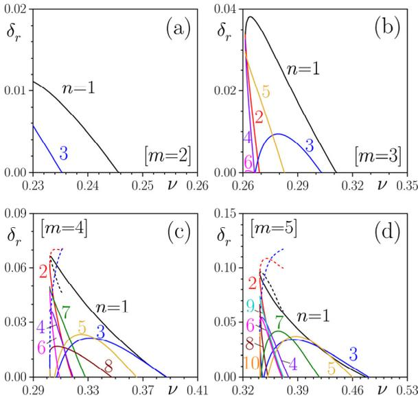
Fig. 3. Real part  $\delta_r$  of perturbation growth rate for different azimuthal perturbation indices  $n$  versus gain amplitude  $\nu$  at  $\alpha = 0.1$  for solitons with  $m = 2$  (a), 3 (b), 4 (c), and 5 (d). Dashed curves in (c),(d) correspond to lower branches of the two-valued  $U(\nu)$  curves.
