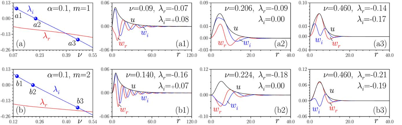
Fig. S1. Real part,  $\lambda_r$ , and imaginary part,  $\lambda_i$ , of the eigenvalue of linear gain-guided mode versus gain amplitude  $\nu$  for topological charges  $m = 1$  (a) and  $m = 2$  (b) at  $\alpha = 0.1$ . Linear mode profiles corresponding to the blue dots in (a) are displayed in (a1-a3) while linear modes corresponding to the blue dots in (b) are displayed in (b1-b3).
