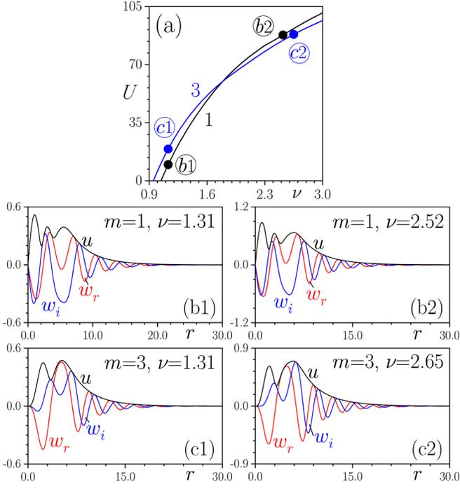
Fig. S4. (a) Norm  $U$  vs pump amplitude  $\nu$  for vortex solitons with topological charges  $m = 1, 3$  at  $\alpha = 0.49$  obtained in the frames of the model (S9). Colored dots and labels next to them correspond to vortex solitons with charges  $m = 1$  (b1),(b2) and  $m = 3$  (c1),(c2). We show both real  $w_r$  and imaginary  $w_i$  parts of the wavefunction, as well as its modulus  $u = (w_r^2 + w_i^2)^{1/2}$ .
