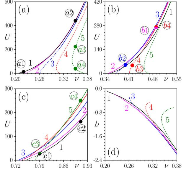
Fig. 1. Energy flow  $U$  vs gain amplitude  $\nu$  at  $\alpha = 0.1$  (a),  $\alpha = 0.2$  (b) and  $\alpha = 0.5$  (c) for vortex solitons with charges  $m = 1, 2, \dots, 5$  indicated next to the curves. (d) Propagation constant  $b$  versus  $\nu$  at  $\alpha = 0.1$ . Stable (unstable) branches are shown with solid (dashed) lines. Colored circles and encircled labels correspond to solitons shown in Fig. 2.
