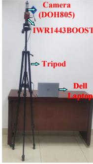
Fig. 15: Hardware platform for data collection.
