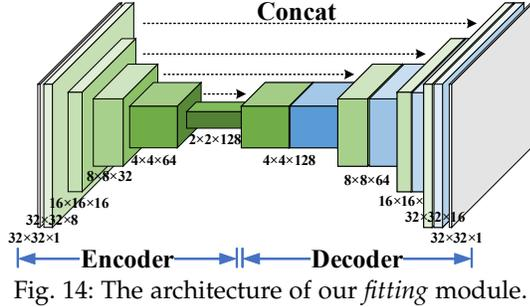
Fig. 14: The architecture of our *fitting* module.
