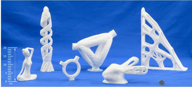
Fig. 13. The results of all models that are fabricated using the support-free curved layers generated by our Neural Slicer.
