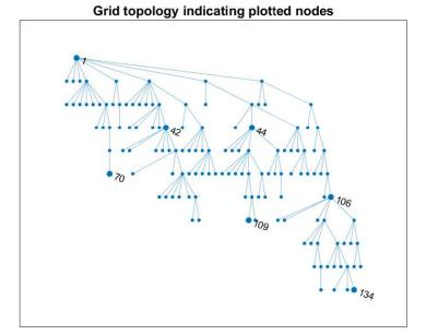
Figure 4: The low-voltage grid topology used in the case-study derived from a real-life Danish 400V grid. The numbered nodes are used later for plots.
