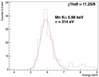
Fig. 4 Low-energy X-ray spectrum obtained with the PT off, prominently featuring the 5.9 keV Mn K- $\alpha$  and 6.4 keV K- $\beta$  (indistinguishable). Notably, the energy resolution at the 5.9 keV Mn K- $\alpha$  peak is measured at 314 ± 22 eV extracted from the fit of the peak with two gaussian to account for Mn K- $\alpha$  and K- $\beta$ .
