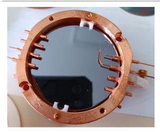
Fig. 1 GaAs detector mounted with PTFE supports on the copper frame. On the right-hand side, the NTD is glued and connected via two 25  $\mu$ m thick gold wires to read the signal. The whole frame was then coupled to the 10 mK stage of the dilution refrigerator.
