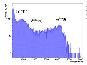
Fig. 3 Energy spectrum of a 12 h calibration with the  $^{238}\mathrm{U}$  Source from 0 to 6 MeV with PT on. This spectrum showcases key radioactive decay events originating from  $^{238}\mathrm{U}$ . It highlights the quenched and degraded  $\alpha$  events peaking at 4198 keV. At lower energy, there are the  $\beta$  decays of  $^{234}\mathrm{Th}$  with an endpoint at 274 keV and  $^{234}\mathrm{(m)}\mathrm{Pm}$   $\beta$  particles, with an endpoint energy at 2290 keV.
