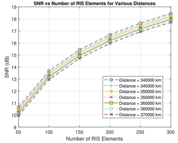
Fig. 5: SNR vs Number of RIS Elements for Various Distances
