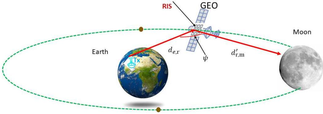
Fig. 1: System Model for a Cislunar Communication Network.
