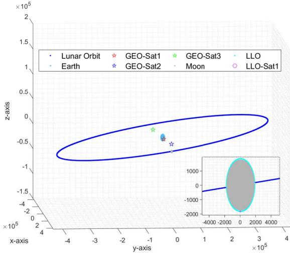
Fig. 2: Time-varying Cislunar system model in the simulation environment.
