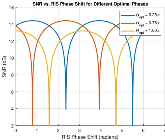
Fig. 4: SNR vs. RIS phase alignment.
