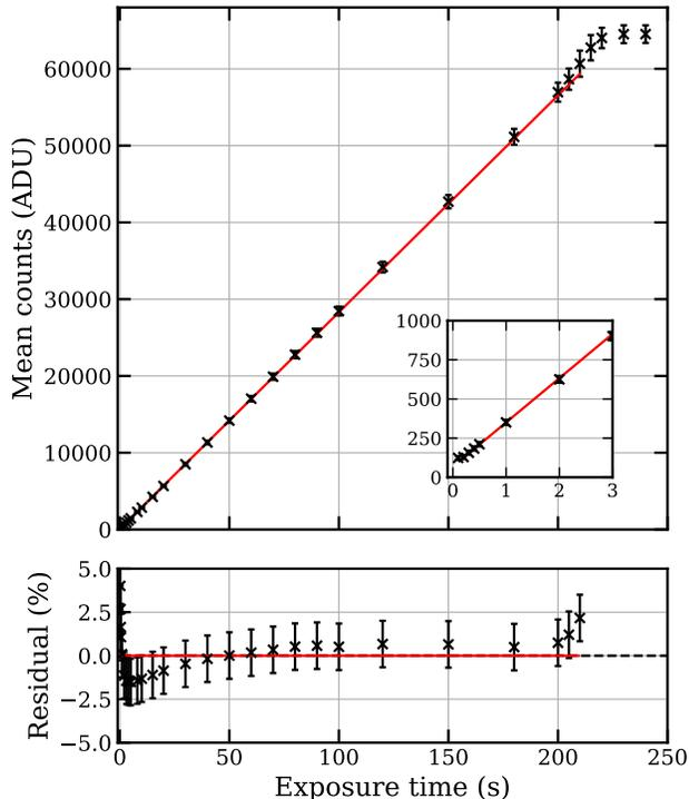
**Figure 3.** The variation of the mean values of the dome-flat images is presented. The linear fit is overplotted in a red solid line from the exposure time of 0.2–210 s. The inset plot shows the linear relation for shorter exposures. The residual plot is also provided in the bottom panel.
