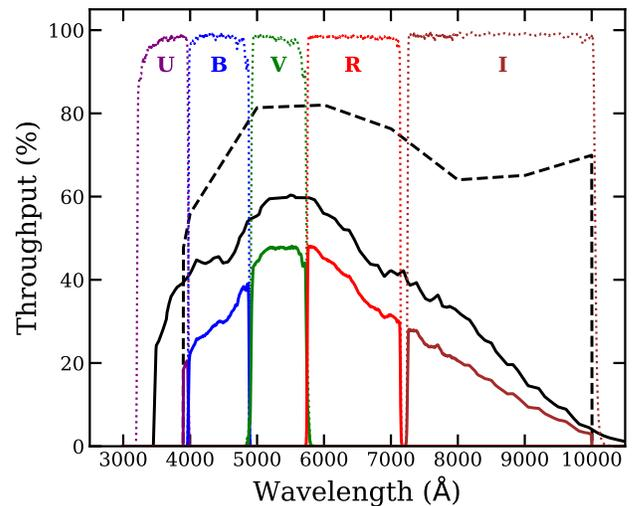
**Figure 5.** Transmission curves of the broadband filter system at MAAO. The optics, CCD QE, and each filter are plotted with black dashed, solid, and dotted lines, respectively. The filter transmission is plotted before and after considering CCD QE and optics (colored solid lines). Note that the *U*-band throughput is not complete since the transmission of the optics and CCD QE is not provided in a wavelength range  $<3900$  and  $<3490$  Å.
