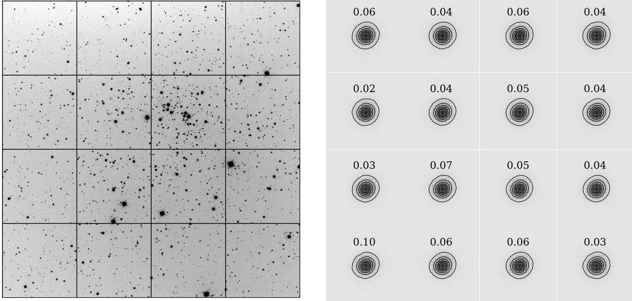
**Figure 8.** Left: The total FOV of the CCD camera for the  $R$ -band image divided into 16 sections. The mean full-width half maximum (FWHM) value in the total field is  $2''.9$  for the 60 s exposure time. Right: PSF images built from stars in each division. The number presents the ellipticity of the PSF.
