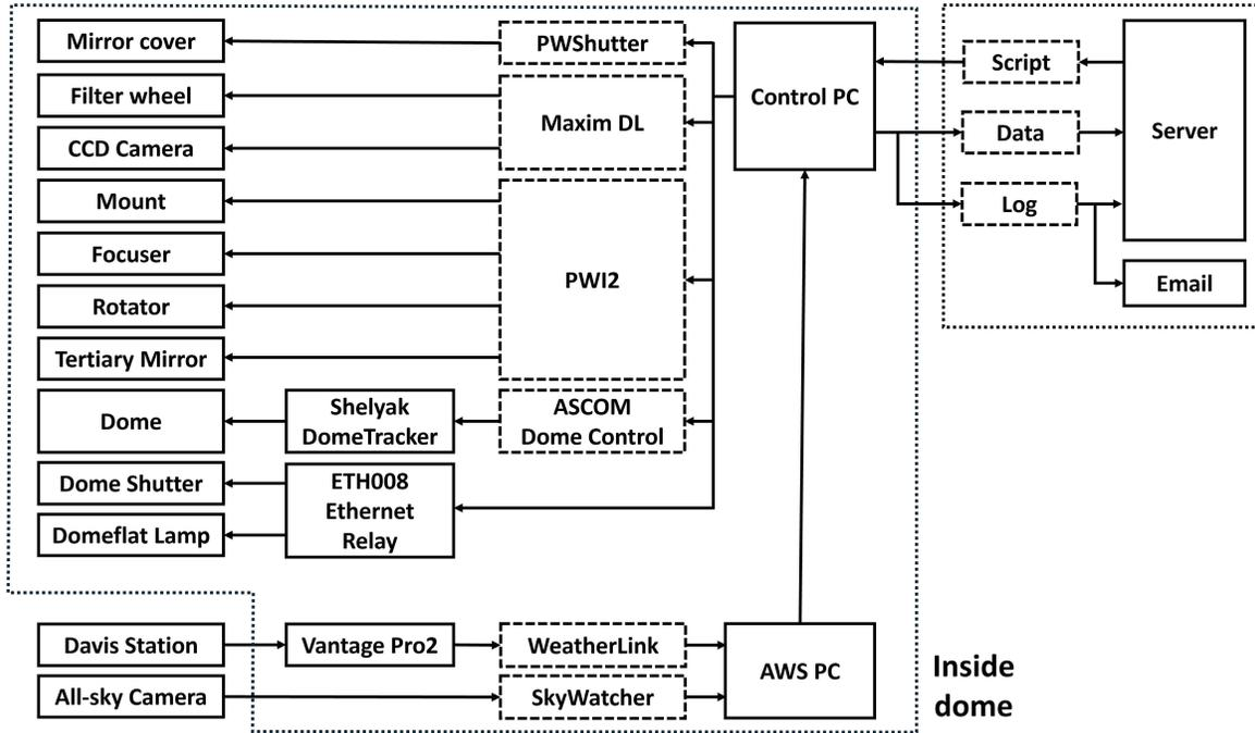
**Figure 6.** A schematic of the system integration at MAAO. Solid boxes represent hardware, while dashed lines indicate computer files and software components, including scripts, data, and logs.
