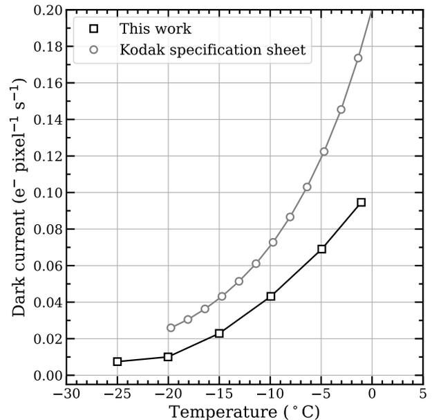
**Figure 4.** A variation of the dark current with the CCD temperature. The data points indicated by gray circles are obtained from the Kodak KAF-16803 Image Sensor Device Performance Specification document (<https://www.onsemi.com/products/sensors/image-sensors/KAF-16801>).
