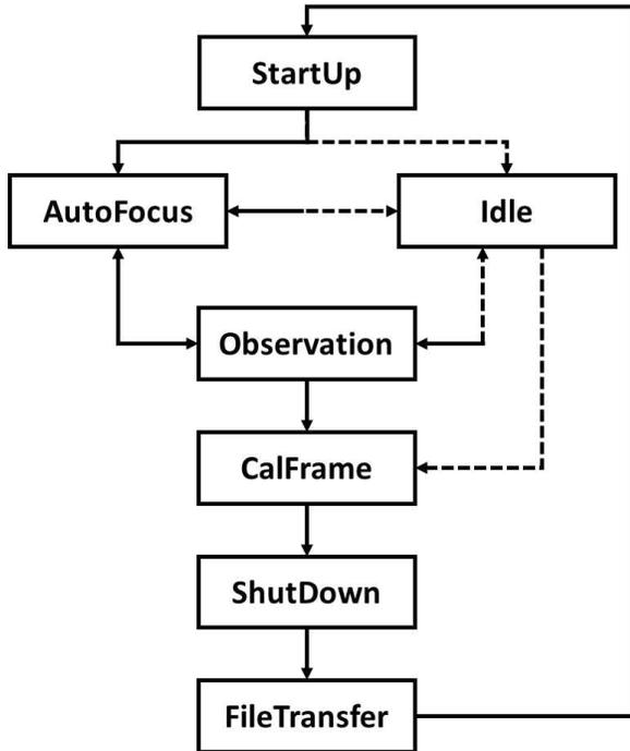
**Figure 7.** A flowchart for the scheduler at MAAO and each session. Solid arrows show the path to the next step when the weather is safe, while dashed arrows represent the path under unsafe weather conditions.
