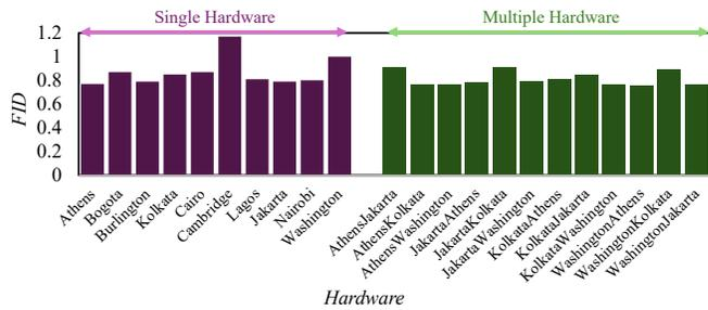
Fig. 5. Plot demonstrating the image quality using FID score for images generated by the qGAN when trained on a single hardware and on multiple hardware.
