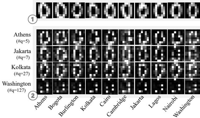
Fig. 6. In this figure (1) shows the original digits dataset with label 0 and (2) shows the images generated qGANs trained on different hardware (along the rows) and inference on 10 IBM backends (along the columns). It can be observed that the noise watermark of the training hardware gets embedded in the images making them visually distinct.
