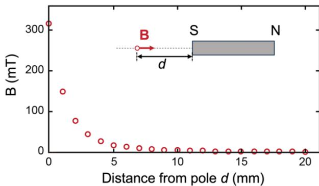
Fig. 6: Measured magnetic flux density  $B$  (mT) of the NdFeB magnet as a function of distance, along the N-S axis, from the one of the poles.
