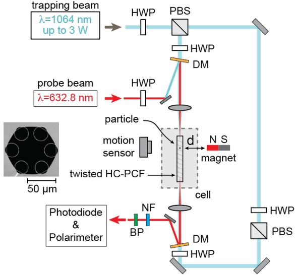
Fig. 2: Schematic of the experimental setup. HWP: half-wave plate, PBS: polarizing beam splitter, DM: dichroic mirror, NF: notch filter at 1064 nm, BP: 1 nm bandpass filter centred at 632.8 nm. The distance between the end of the magnet and the fibre is  $d$ . Inset: Scanning electron micrograph showing the cross-section of the single-ring HC-PCF. The core diameter of the fiber is  $44 \mu\text{m}$  and the outer diameter  $\sim 270 \mu\text{m}$ . The motion sensor is a quadrant photodiode.
