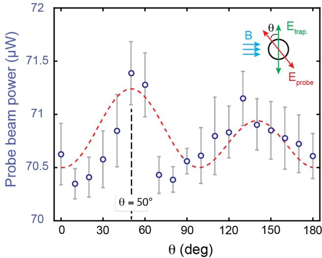
Fig. 4: Transmitted probe power as the particle is rotated inside the HC-PCF and subject to a constant magnetic field of 29 mT. The red dotted curve is a heuristic fit to Eq. (3).
