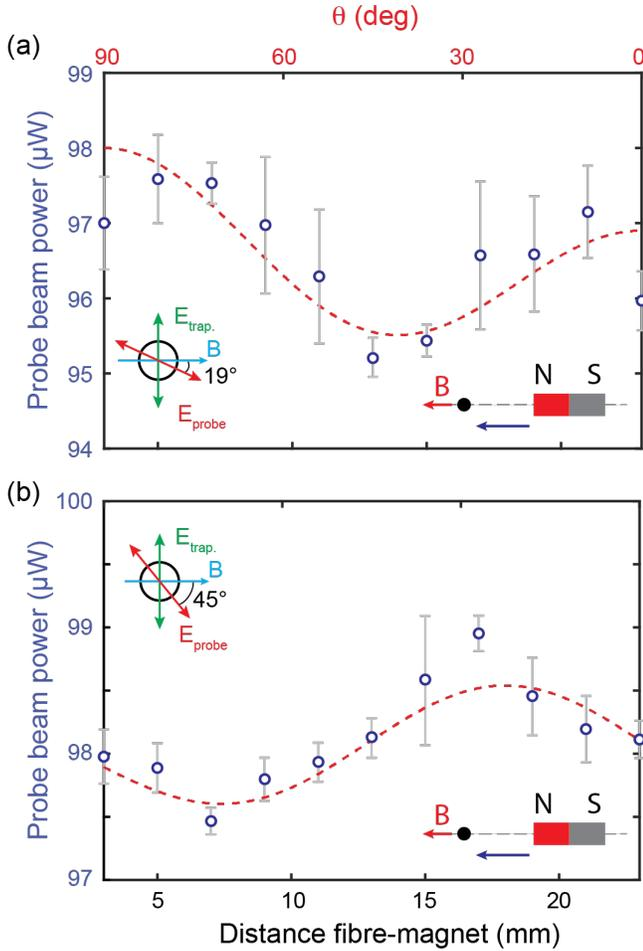
Fig. 5: Transmitted power (blue axis) as the magnet is moved inwards towards the particle. The angle between the orientation of the linearly polarized probe beam and the applied external field  $B$  is  $19^\circ$  in (a) and  $45^\circ$  in (b). The red dashed line is a heuristic fitting using Eq. (3)
