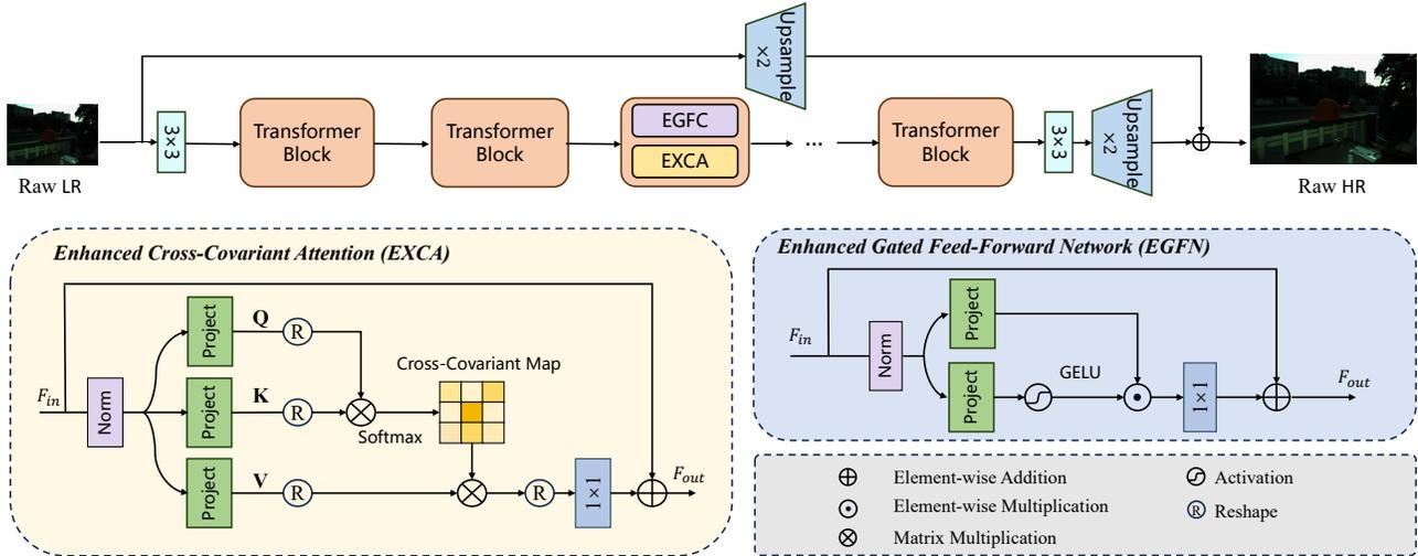
Figure 5. The RBSFormer [25] Framework proposed by Team USTC604.
