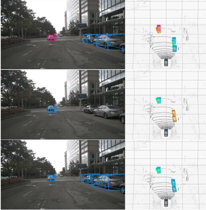
Figure 11: Corner case example for camera, radar and fusion models respectively from top to bottom. Same bounding box color coding as in Figure 10. Even when single-sensor models fail to predict all objects in the scene, a fusion model utilizes both sensors’ data to improve upon each of them.
