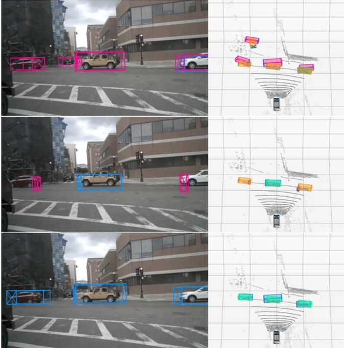
Figure 10: Prediction results for the same test dataset scene for camera-only, radar-only and CDMS fusion models respectively from top to bottom. On both images and corresponding 3D views, we marked predicted bounding boxes matched as true positives (predictions in blue, matched targets in green), false detections (magenta) and missed objects (yellow). LiDAR pointcloud added for reference in BEV view.
