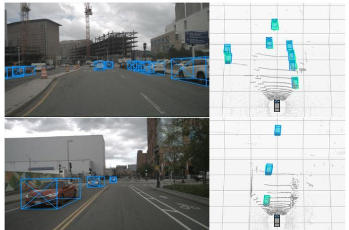
Figure 2: Example results of CDSM fusion method predictions on NuScenes test data. Predicted objects are marked in blue, both in a camera and an enhanced BEV view. Green cuboids represent matched groundtruth labels. LiDAR pointcloud added for reference in BEV view.
