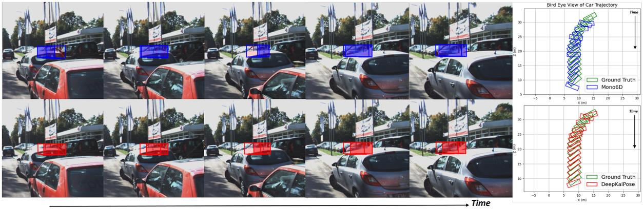
**Fig 3** Qualitative results demonstrating improved car trajectory estimation on an occluded and distant vehicle. The sequence displays the projected 3D bounding boxes: the upper row illustrates results from Mono6D [1], while the lower row illustrates results from our proposed methodology. The two figures on the extreme right detail the temporal Bird's Eye View (BEV) comparison between the 3D BB estimations by Mono6D and DeepKalPose, respectively.
