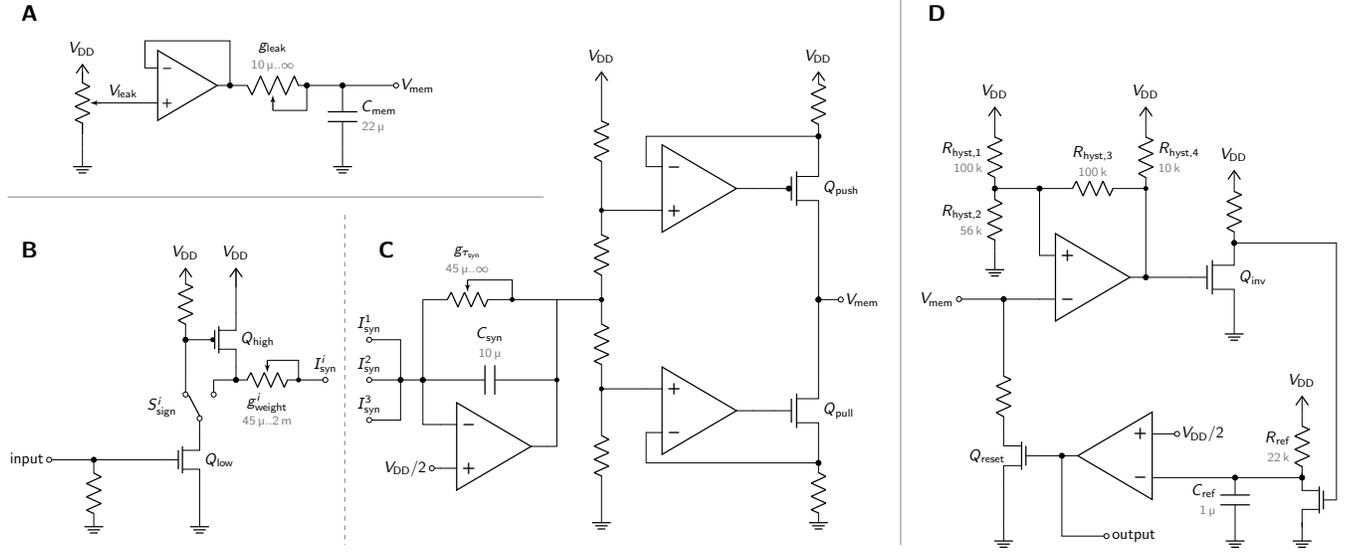
**Figure 2.** Schematic of the LIF emulation circuit implemented in Lu.i. (A) Membrane capacitance and leakage resistance. (B) Current-based synaptic input circuits. This circuit is instantiated three times, once per synapse. (C) Synaptic integrator and voltage-to-current conversion circuit. (D) Threshold, reset, and refractory circuit. The spike output pulse is derived from the neuron’s reset signal and of equivalent duration.
