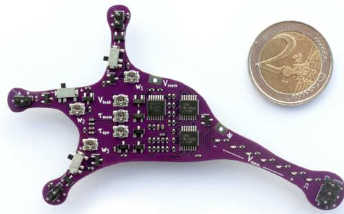
**Figure 1.** A single Lu.i neuron PCB, with a 2-Euro coin for scale. To relay information from one neuron to the other, excitatory and inhibitory synapses can be formed by wiring the axonal output (right) to one of the three dendritic terminals (left).
