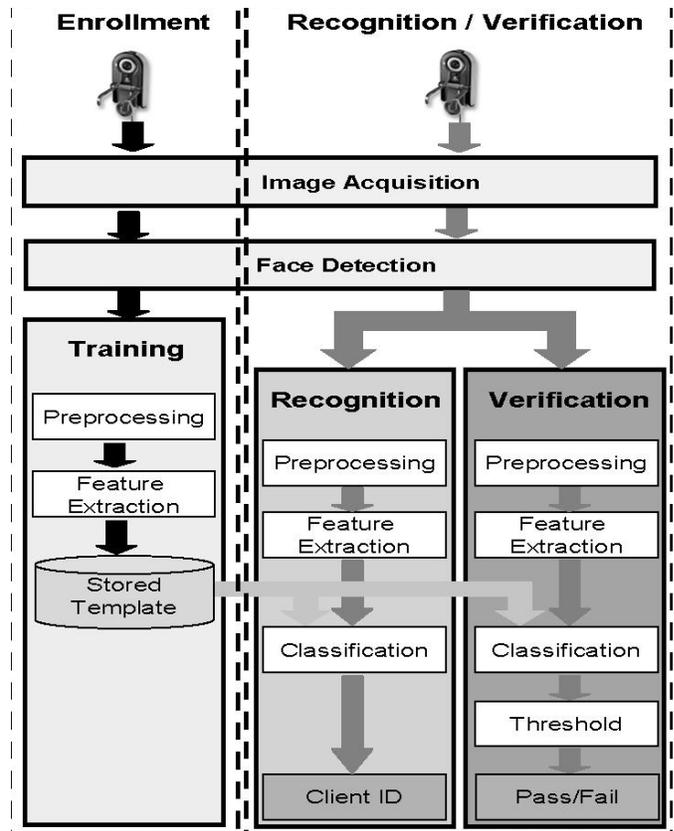
Figure 5. Block Diagram for the Face Recognition System [5]
