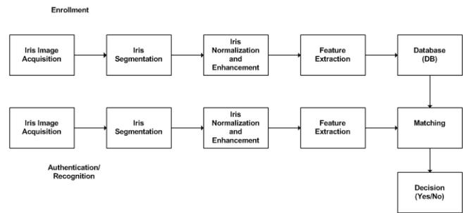
Figure 9. Generalized Block Diagram of Iris Recognition System.
