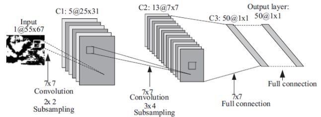
Figure 8. Proposed CNN architecture
