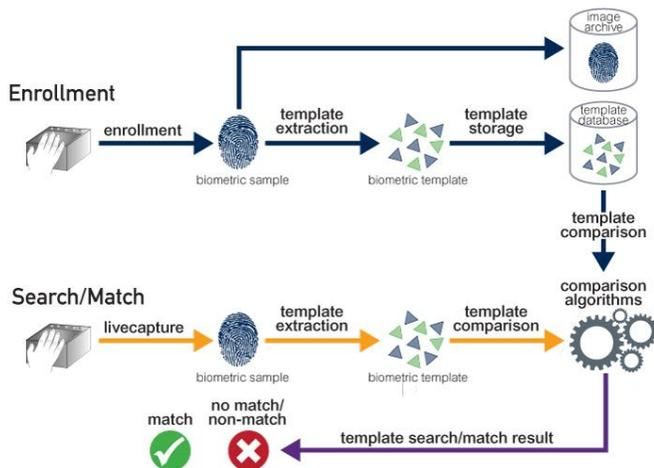
**Figure 1. 3 steps in Biometric Recognition**
