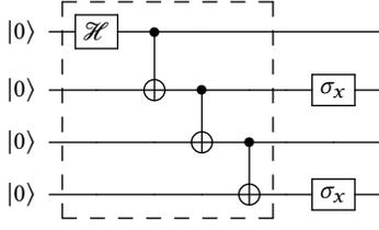
**Figure 4: Quantum circuit of  $\mathcal{E}(\{1, -1, 1, -1\})$  applied to  $|0\rangle^{\otimes 4}$ .** The section outlined by dash line prepares a 4-qubit GHZ state [28], while the following  $\sigma_x$  gates conduct bit-flipping.
