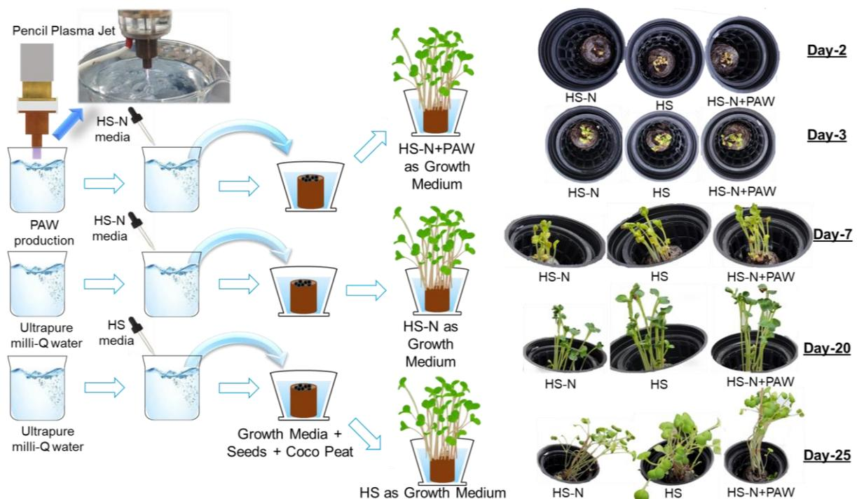
**Figure 1.** Schematic of the use of plasma-activated water (PAW) as a nitrogen source for hydroponic solution (HS) as the growth medium for radish plants. HS-N: hydroponic solution without nitrogen, HS-N+PAW: hydroponic solution with PAW as the nitrogen source.
