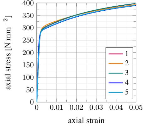
Figure 8: Stress-strain data for calibration
