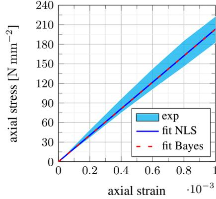
Figure 9: Experimental and calibrated stress-strain data in the elastic domain
