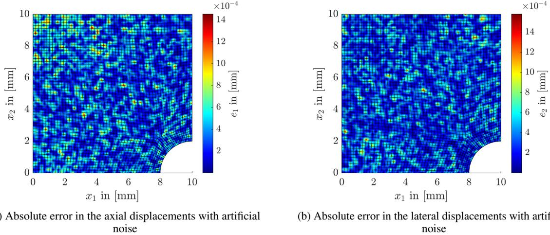
Figure 6: Absolute error between generated displacements with  $\mathcal{N}(0, (4 \times 10^{-4} \text{ mm})^2)$  and computed displacements with the identified parameters in the NLS scheme with FEM
