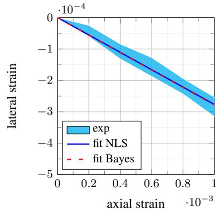
Figure 10: Experimental and calibrated lateral strain data in the elastic domain
