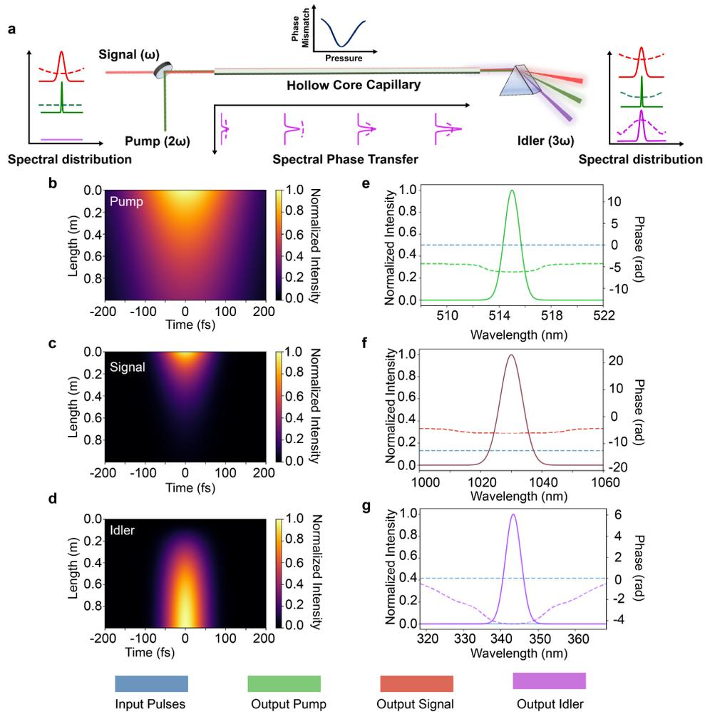
Figure 1. (a) Schematic of FWM in a gas-filled HCC. The optimal phase match condition (inset) can be achieved with Ar at room temperature, approximately at 0.63 bar. (b-d) Temporal intensity evolution of pump, signal and idler pulses (x-axis) as they propagate along (y-axis) the Ar-filled hollow core capillary. (e-g) Comparative analysis of the input and output spectra, along with the phase of the pump, signal, and idler pulses, respectively.
