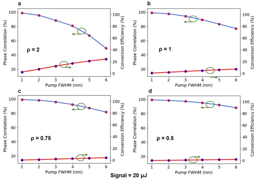
Figure S3. The interplay between efficiency, measured as the  $\Delta\lambda_p$  (FWHM) of the pump spectrum, and the phase quality, represented by the linearity of the idler pulse with  $\rho = 2$ ,  $\rho = 1$ ,  $\rho = 0.75$  and  $\rho = 0.5$ . The signal pulse energy is fixed at 20 μJ.
