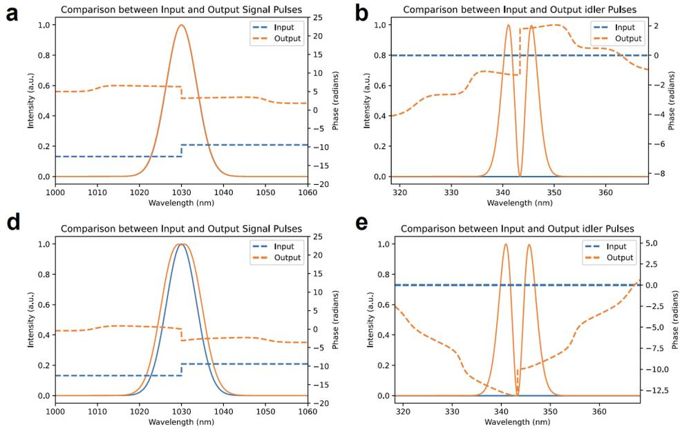
Figure S4.  $\pi$ -step phase transfer. (a-b) focused on better phase transfer from the signal (a) to idler (b) with  $\rho = 1$ . (c-d) focused on higher conversion efficiency signal (a) to idler (b) with
