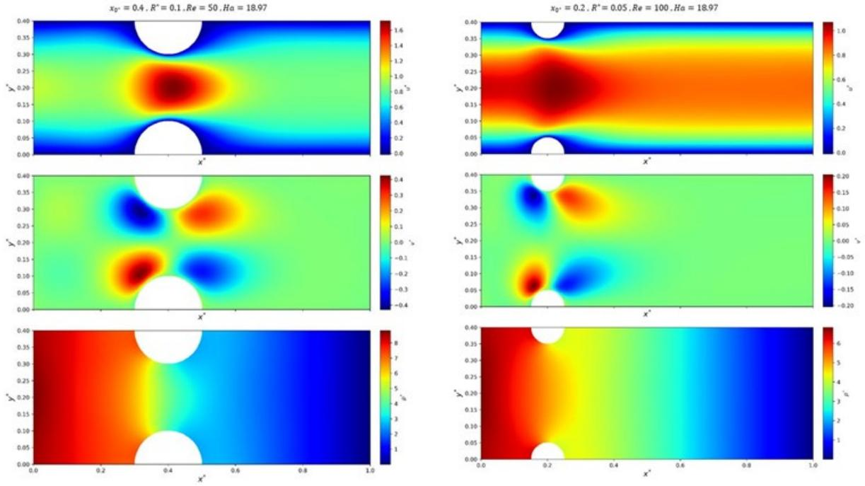
Figure 8: Contours of dimensionless velocity components and pressure when magnetic fields are applied, obtained from PINN
