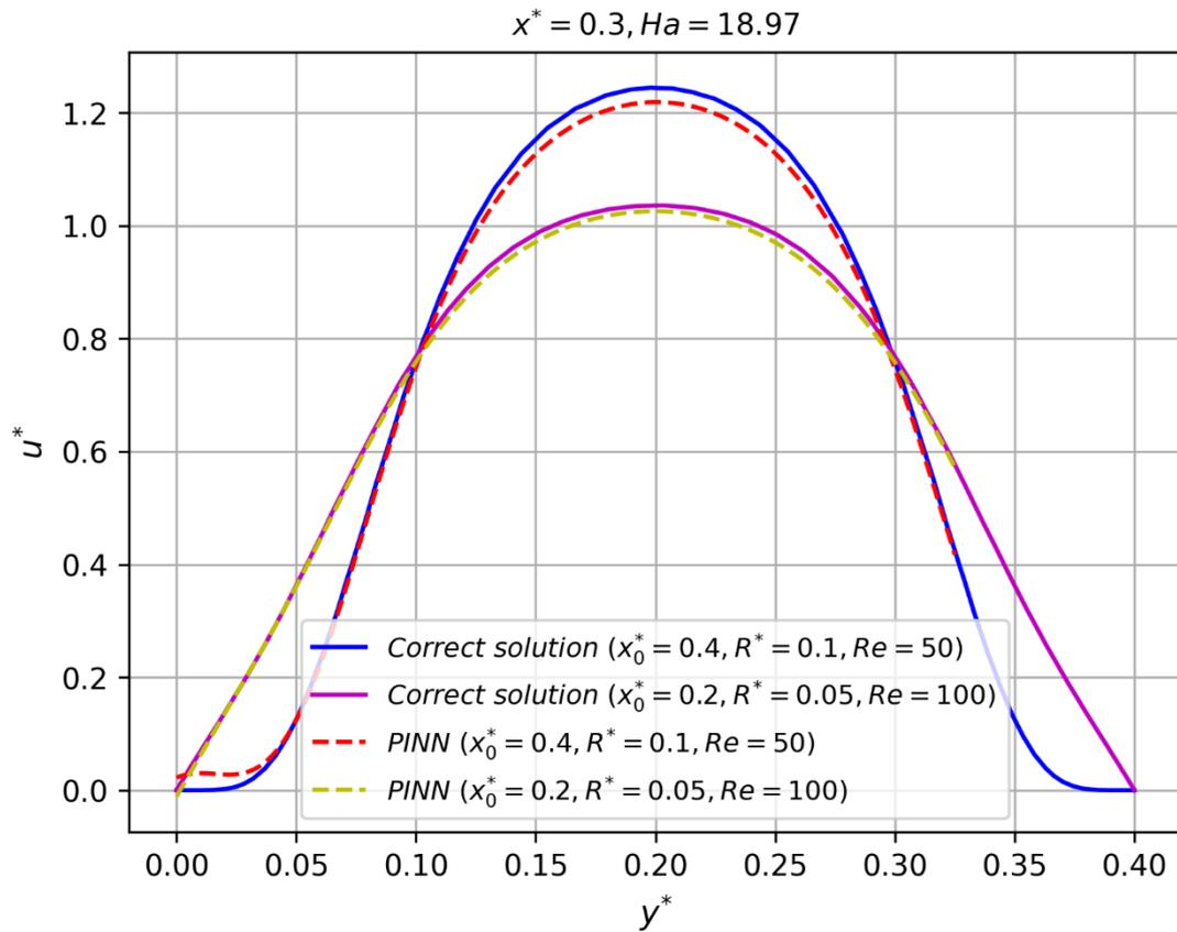
Figure 10: changes of the dimensionless velocity component in x direction in a section of the channel and comparison with the correct results for the flow under the influence of magnetic field
