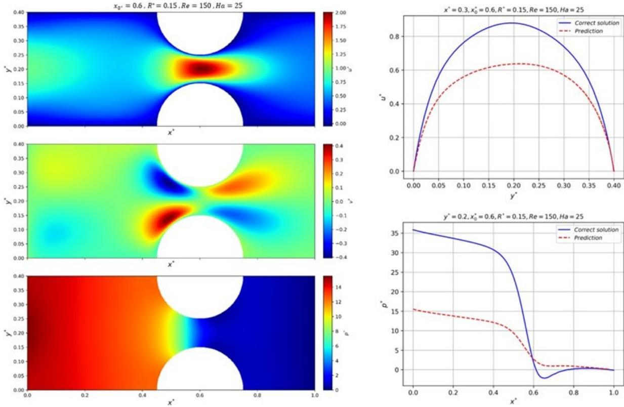
Figure 11: Comparing results calculated by PINN with the correct results
