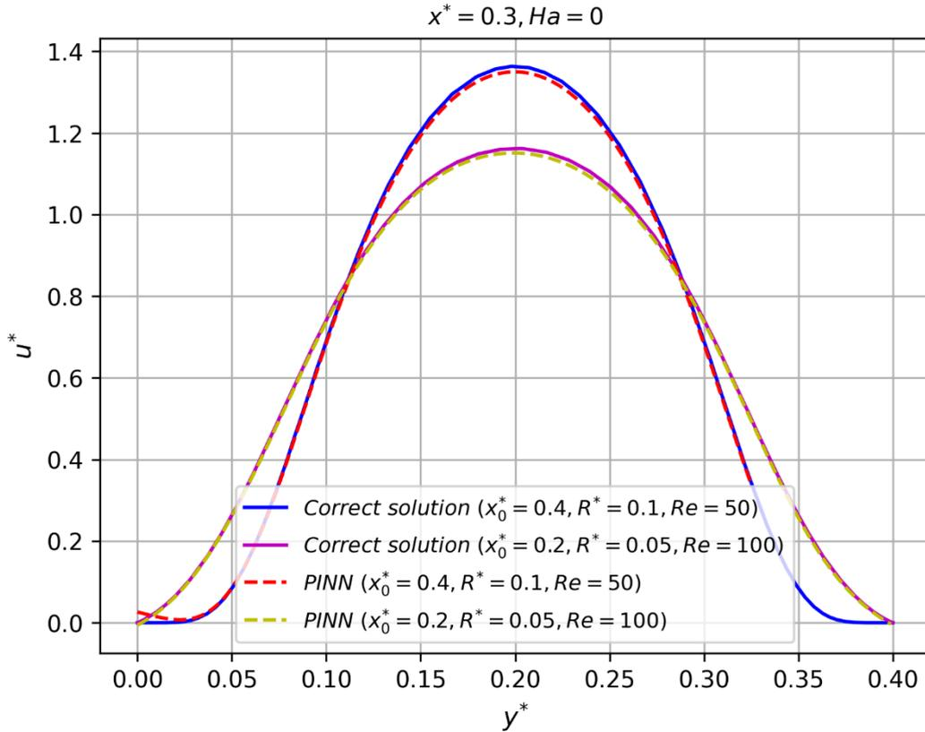
Figure 7: Comparison of the velocity component in x direction in a section of the channel obtained by PINN and the correct results.
