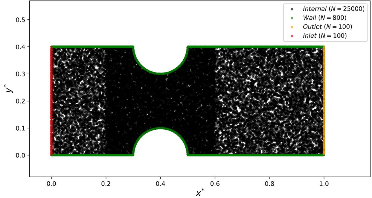
Figure 3: Points generated using LHS method for use in governing equations and boundary conditions
