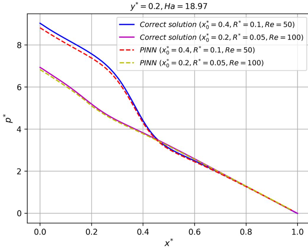
Figure 9: Comparing dimensionless pressure changes along the centerline of the channel with correct results of flow influenced by magnetic fields
