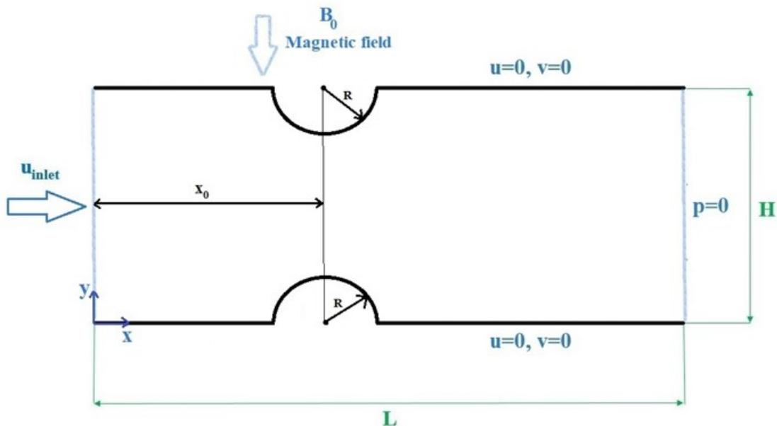
Figure 1: Geometric specifications and boundary conditions
