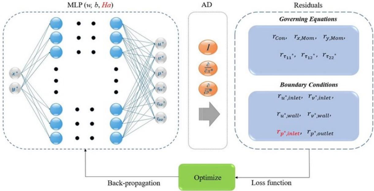
Figure 13: Schematics of the physics informed neural network used to solve the inverse problem
