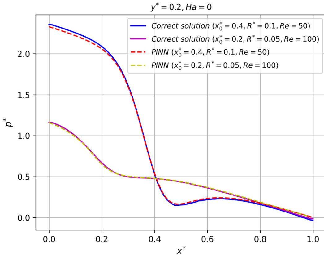
Figure 6: Trend of dimensionless pressure along the centerline of the channel and comparison with correct results.
