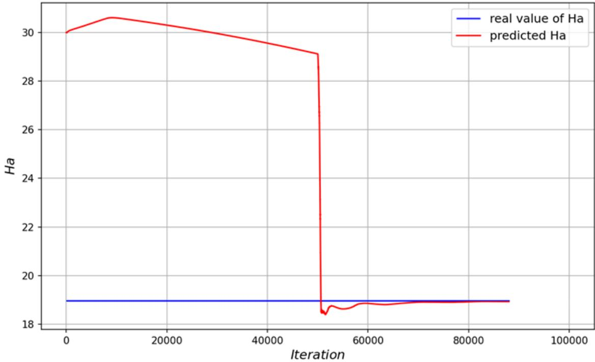
Figure 14: Calculated Hartmann number as the training process progressed
