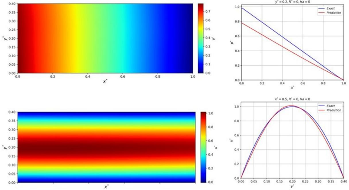
Figure 12: Comparison of the results obtained from PINN with analytic solution of the Poiseuille flow
