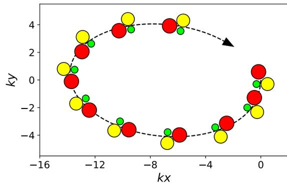
FIG. 3. Simulated dynamics of three dense spheres starting from rest in the nodal plane of a planar standing wave. The cluster is bound by conservative König interactions as it traces out an ellipse and rotates about its center of mass under the influence of nonreciprocal pair interactions and viscous drag.
