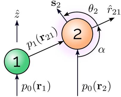
FIG. 1. Geometry for computing the wave-mediated forces. Particle 1 scatters a portion of the incident sound wave to its neighbor at  $\mathbf{r}_2$ . The scattered wave interferes with the incident wave and therefore influences the force experienced by particle 2. Formulating this influence is facilitated by defining a spherical coordinate system centered on particle 2 and aligned with the separation between the particles,  $\mathbf{r}_{21} = \mathbf{r}_2 - \mathbf{r}_1$ .
