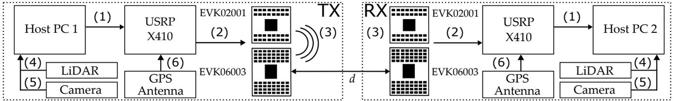
Fig. 1: Schematic of the multi-band mm-wave measurement platform with connection types and signals: (1) samples, (2) I-Q baseband signal (bandwidth support up to 400 MHz), (3) RF signal ( $f_c = 28/60$  GHz), (4)  $2048 \times 128$  point cloud, (5)  $360^\circ$  video stream, (6) 3D position (latitude, longitude and altitude).
