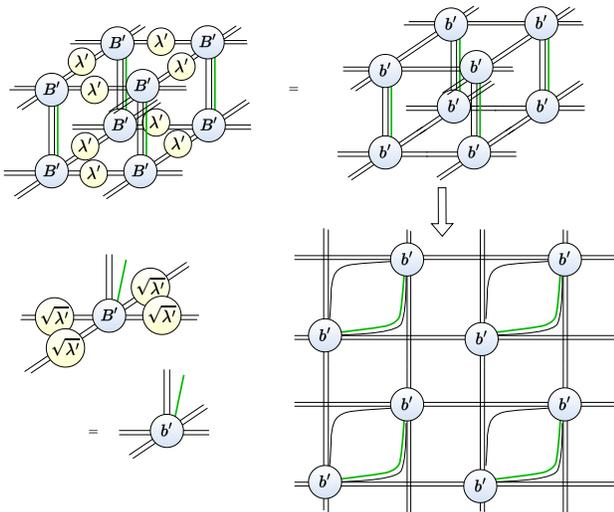
FIG. 7. The mapping of the non-reduced two-layer tensor network with the  $1 \times 1$  unit cell to the single-layer tensor network with the  $2 \times 2$  unit cell. The mapping also introduces auxiliary tensors, which consist only of the products of the Kronecker deltas.
