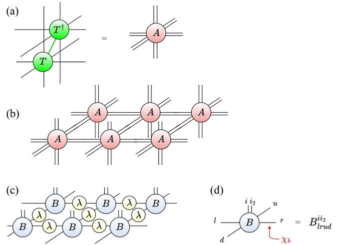
FIG. 3. (a) Definition of the double-layer tensor  $A$  and (b) infinite 3d tensor network composed of these tensors (the transfer matrix  $M$  consists of all tensors  $A$  on the horizontal plane); (c) The left boundary PEPS (bPEPS) consists of identical tensors  $B$  and positive matrices  $\lambda$  placed on its virtual links. (d) Each tensor  $B$  has the bond dimension  $\chi_b$  for its four virtual indices.
