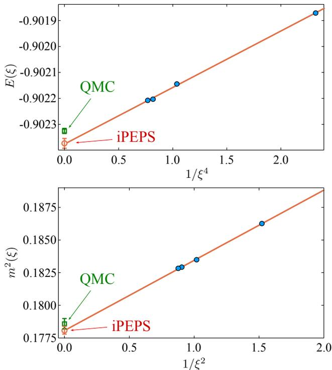
FIG. 11. Dependence of the energy  $E(\xi)$  and square of magnetization  $m^2(\xi)$  per site obtained with iPEPS for  $D \in [4, 7]$  (circles) with the corresponding linear fits to the powers of the correlation length  $\xi^{-4}$  and  $\xi^{-2}$ , respectively. The estimated extrapolated values (open circles with error bars) are  $E = -0.90237(2)$  and  $m^2 = 0.1781(3)$ . QMC data points (open squares with error bars) are taken from Ref. [44].
