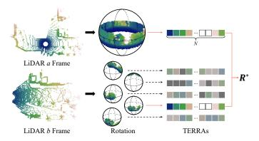
Fig. 5. Instructions for rotation initialization. Each LiDAR frame has a TERRA extracted from it. Then the descriptor of one LiDAR is fixed, while rotating the other to find the optimal match. The rotation corresponding to the optimal match is the result of the rotation initialization. Different colors represent different values and the TERRA is a vector of length N.
