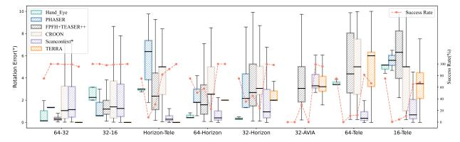
Fig. 11. The rotation error and success rate of rotation initialization tasks. We select eight representative LiDAR pairs from the COLORFUL dataset for calibration and test six methods. The x-axis of the graph represents the LiDAR types involved in the eight calibration tasks. The box plot indicates rotation error, while the line graph represents the success rate.
