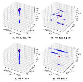
Fig. 15. Rotations and their corresponding distances. The axes represent the Euler angles for rotation around the x, y, and z axes, respectively. The opacity signifies the value of the distance, where less opacity indicates a smaller distance. The red point represents the location of the ground truth. ED is an abbreviation for Euclidean Distance.
