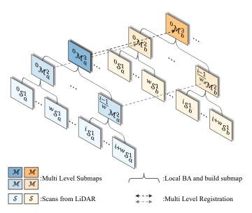
Fig. 8. Hierarchical optimization for pose refinement. Each LiDAR constructs local maps at different levels and optimizes the pose through local LiDAR BA with in the same window.
