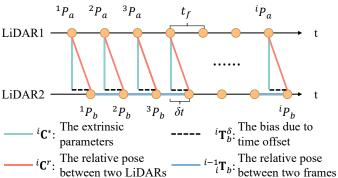
Fig. 9. The estimated extrinsic is disturbed by motion due to time offset. We identify the optimal extrinsics by determining the time offset.
