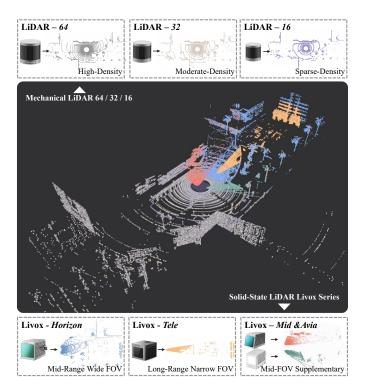
Fig. 1. The illustration of seven types of LiDAR in the simulated dataset. Mechanical LiDARs exhibit varying densities, solid-state LiDARs have different FOV, and mechanical and solid-state LiDARs have distinctly different point cloud distributions. This diversity presents new challenges for LiDAR calibration. This paper aims to introduce a universal, sensor-agnostic calibration method.
