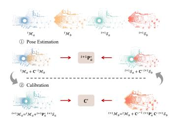
Fig. 7. Instructions for JEEP. For point cloud pairs input at the same time, their transformation relative to the map, i.e., poses, and the transformation between them, i.e., extrinsic, are iteratively solved until either convergence is achieved or a convergence failure is indicated by the number of iterations.
