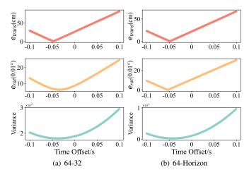
Fig. 19. The relationship between the sampled time offset and extrinsic variance. The ground truth time offset is -50ms.
