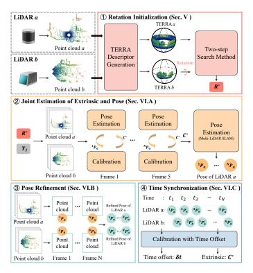
Fig. 2. The pipeline of the universal LiDAR calibration involving four core steps, i.e., TERRA based rotation initialization, JEEP for joint estimation of extrinsic and poses, hierarchical optimization based pose refinement and time synchronization for enhancing the accuracy of extrinsic parameters and estimating the time offset.
