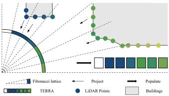
Fig. 4. Instructions for the generation of TERRA. The process is divided into three steps: sampling the sphere using the Fibonacci lattice, projecting the point cloud from LiDAR onto the unit sphere, and populating the values into TERRA based on the correspondences.
