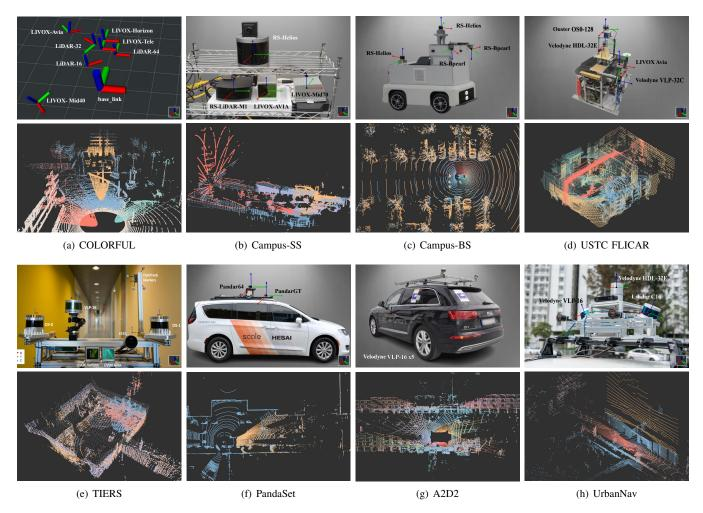
Fig. 10. The platform and point clouds of utilized datasets. Three datasets are self-collected, five are publicly available; one is a simulated dataset, and seven are real-world datasets. These encompass 16 diverse types of LiDAR. For each dataset, the upper figure represents the actual position of the LiDARs, and the lower one illustrates the calibrated point clouds from LiDARs.
