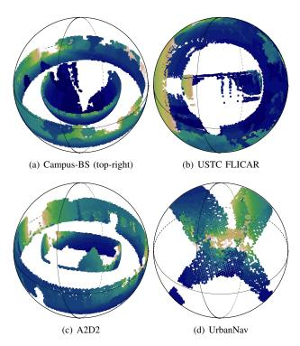
Fig. 13. The challenging example of the TERRA in the real-world dataset. The TERRA for the first LiDAR is represented by the outer sphere, while the second is illustrated by the inner sphere. For UrbanNav, both spheres are the same size.
