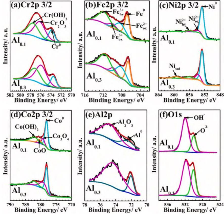
**Figure 2.** XPS results of O 1s, Cr 2p<sub>3/2</sub>, Fe 2p<sub>3/2</sub>, Co 2p<sub>3/2</sub>, Ni 2p<sub>3/2</sub> and Al 2p for the surface film formed upon following exposure to 0.5 M H<sub>2</sub>SO<sub>4</sub> – for FeCoCrNiAl<sub>x</sub> (where x = 0.1 or 0.3, as depicted in the figure) [34]
