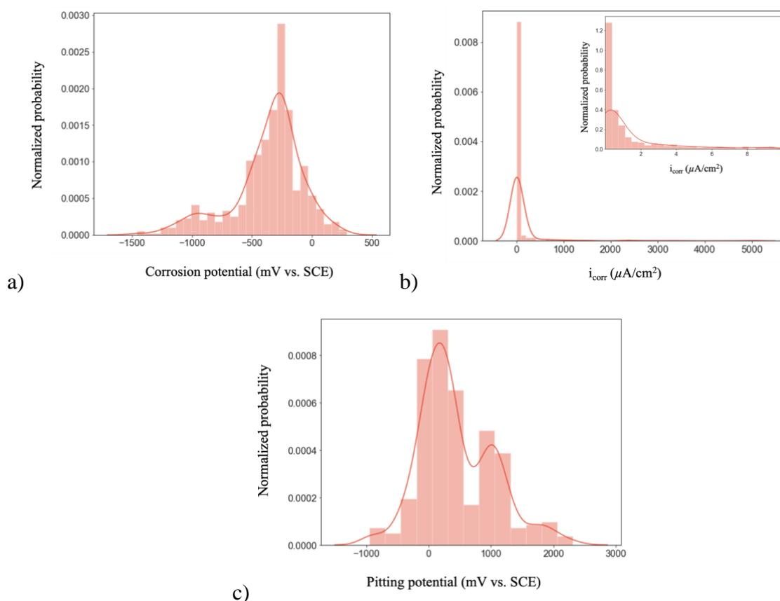
**Figure 5.** Data distributions for corrosion related parameters of alloys in the MPEA corrosion database, showing a) corrosion potential, b) corrosion current density, and c) pitting potential.
