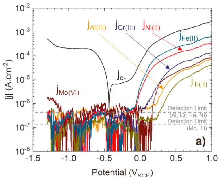
**Figure 1.** Equivalent current densities of in-situ elemental dissolution rates monitored via ASEC during polarization of the base alloy of  $Al_{0.3}Cr_{0.5}Fe_2Mo_xNi_{1.5}Ti_{0.3}$  with 3.2 at. % Mo in nitrogen sparged 0.1 M NaCl (pH 4). Dashed lines indicate element detection limits.
