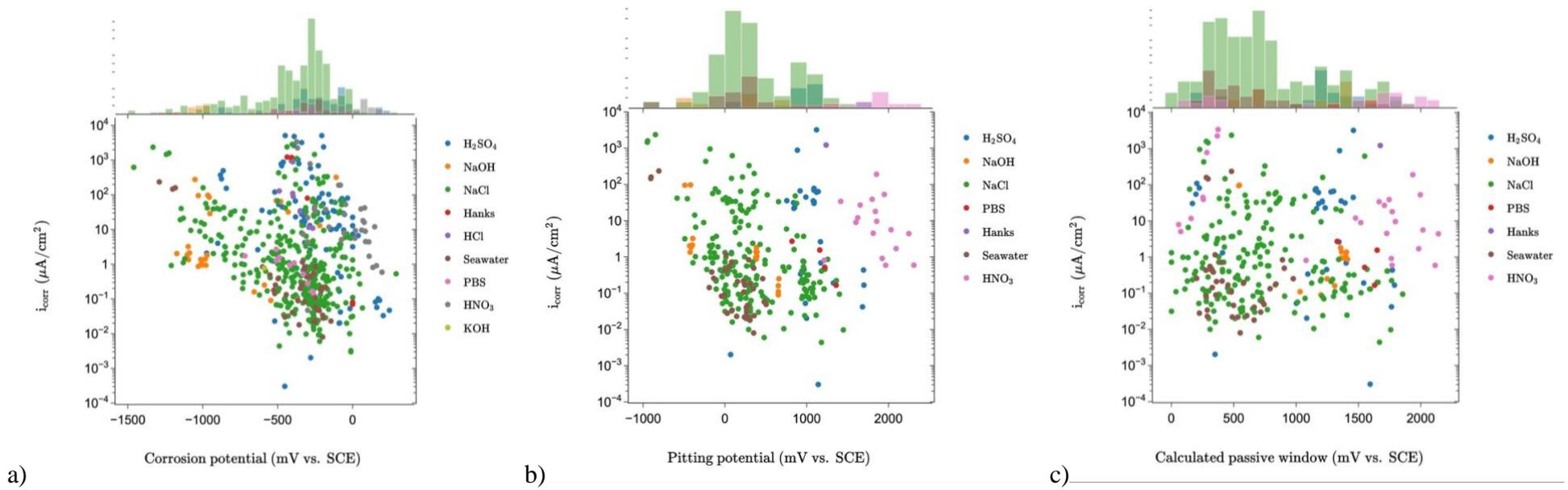
**Figure 6.** The corrosion current density data versus the corresponding a) corrosion potential, b) pitting potential, and c) calculated passive window for alloys in the MPEA corrosion database, with data disambiguated by test electrolyte. Additionally, the univariate distribution of the parameter represented by the x-axis is shown in the top margin of each plot.
