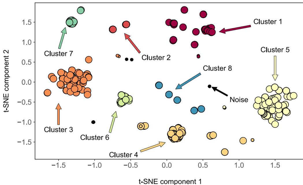
**Figure 10.** DBSCAN clustering analysis in combination with t-SNE dimension reduction algorithm revealing eight distinct clusters separated based on the similarities in the MPEA corrosion database.
