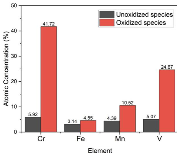
**Figure 3.** Atomic concentration of unoxidized and oxidized species on the surface of CrFeMnV as determined using XPS, after 1 h immersion in 0.6 M NaCl. [27]
