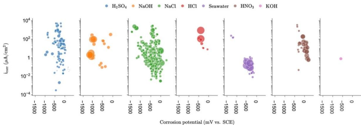
**Figure 7.** The role of the test electrolyte on the reported corrosion potential and corrosion current density for alloys in the MPEA corrosion database. The size of the datapoints represents the relative concentration of the test electrolyte.
