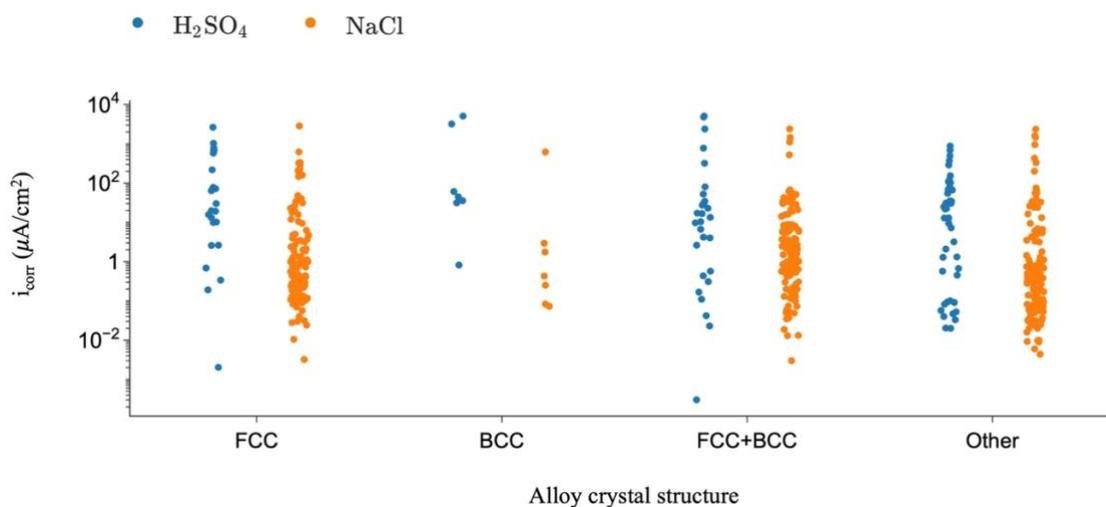
**Figure 9.** MPEA crystal structure reported versus the corresponding corrosion current density data for all alloys in the MPEA corrosion database. Data is presented for the two most prevalent test electrolytes,  $\text{H}_2\text{SO}_4$  and NaCl.
