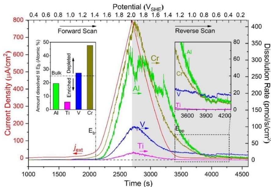
**Figure 4.** ASEC cyclic polarisation curve of AlTiVCr showing incongruent dissolution in dilute NaCl, during a forward and reverse potential scan. Significant enrichment of Ti on the alloy surface occurs, resulting in the rapid re-passivation during the reverse potential scan.  $E_b$  and  $E_{pp}$  represent final breakdown potential and protection potential, respectively [19].
