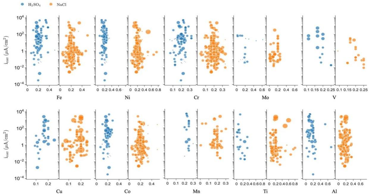
**Figure 8.** The relationship between the corrosion current density and the alloy fraction of the most important alloying elements in MPEAs (represented by atomic fraction), including Fe, Ni, Cr, Mo, V, Cu, Co, Mn, Ti, and Al. The data has been presented in a manner that prioritises (and separates) the two most prevalent test electrolytes,  $H_2SO_4$  and NaCl. The size of the datapoints represents the relative concentration of the test electrolyte.
