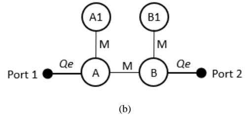
Fig. 3. Filter coupling arrangements (a) single-band, (b) dual-band.
