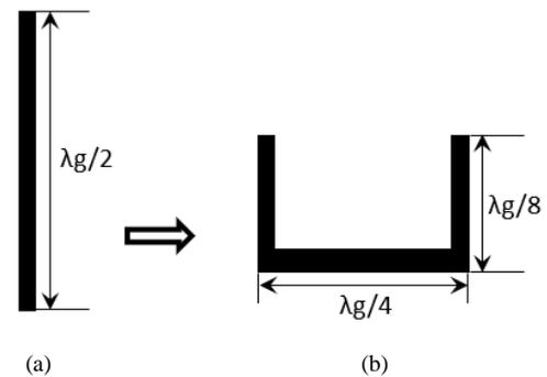
Fig. 1. Resonator configurations (a) half-wavelength, (b) U-shaped.
