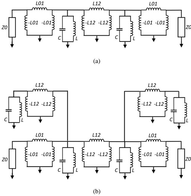
Fig. 2. Filter circuit configurations (a) single-band, (b) dual-band.
