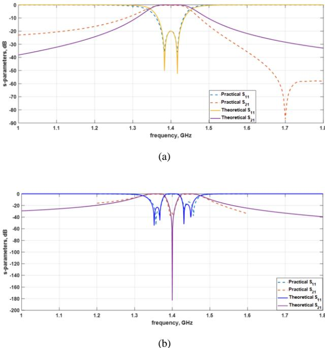
Fig. 6. Theoretical and practical filter results comparison (a) single-band, (b) dual-band.
