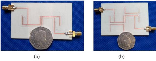
Fig. 5. Fabricated filter image (a) single-band, (b) dual-band.
