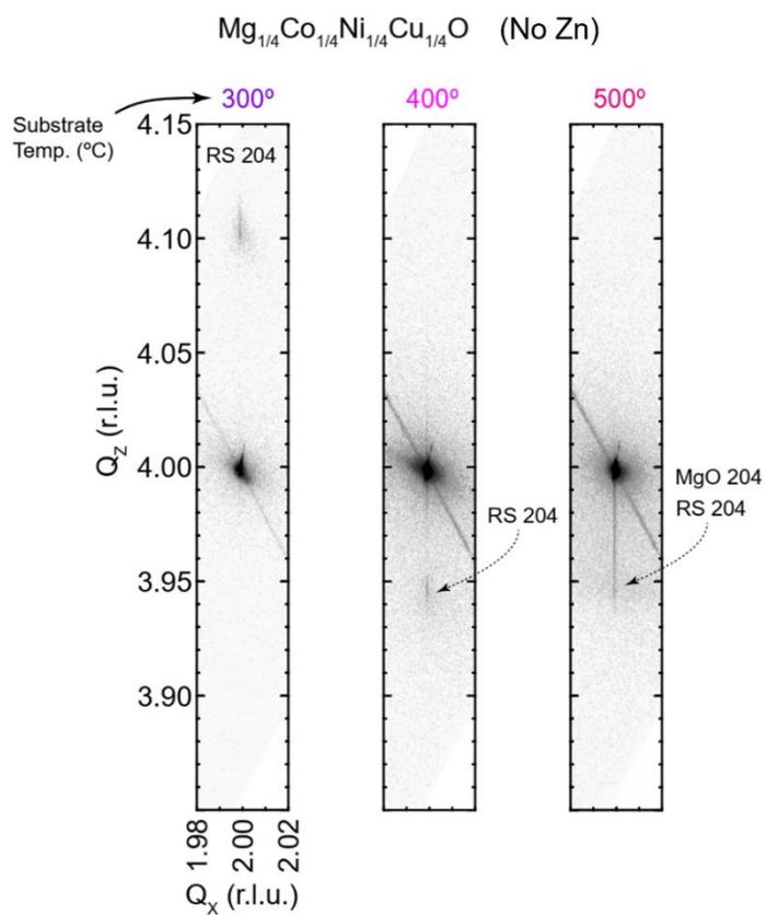
**Figure S11.** Reciprocal space maps of  $\text{Mg}_{1/4}\text{Co}_{1/4}\text{Ni}_{1/4}\text{Cu}_{1/4}\text{O}$  (No Zn) and MgO 204 reflections, indicating commensurate film growth. Substrate temperature during film growth is indicated near each plot.
