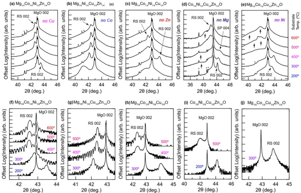
**Figure 4.** X-ray diffraction patterns of  $\text{Mg}_{1/5}\text{Co}_{1/5}\text{Ni}_{1/5}\text{Cu}_{1/5}\text{Zn}_{1/5}\text{O}$  and four-component derivative thin films. (a-e) are low resolution scans with divergent beam for all films grown at temperatures 200 °C to 600 °C and (f-j) are higher resolution scans with parallel beam for only single phase films. Asterisks indicate  $\text{Cu}\beta$  and W reflections.
