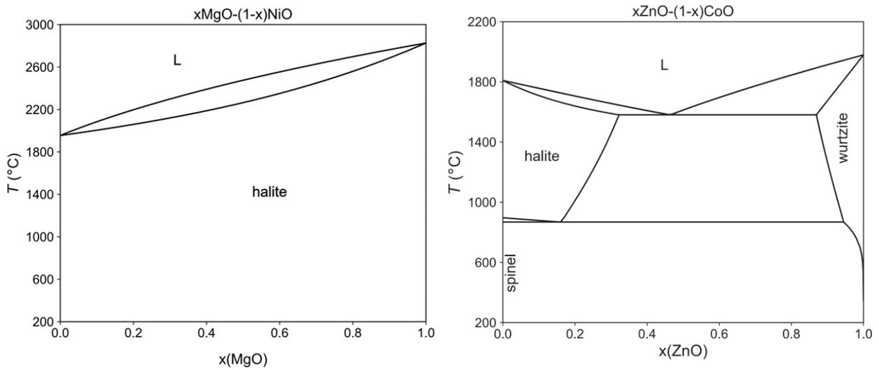
**Figure S2.** Binary phase diagrams for MgO and NiO with complete solubility and CoO and ZnO with no apparent solubility.
