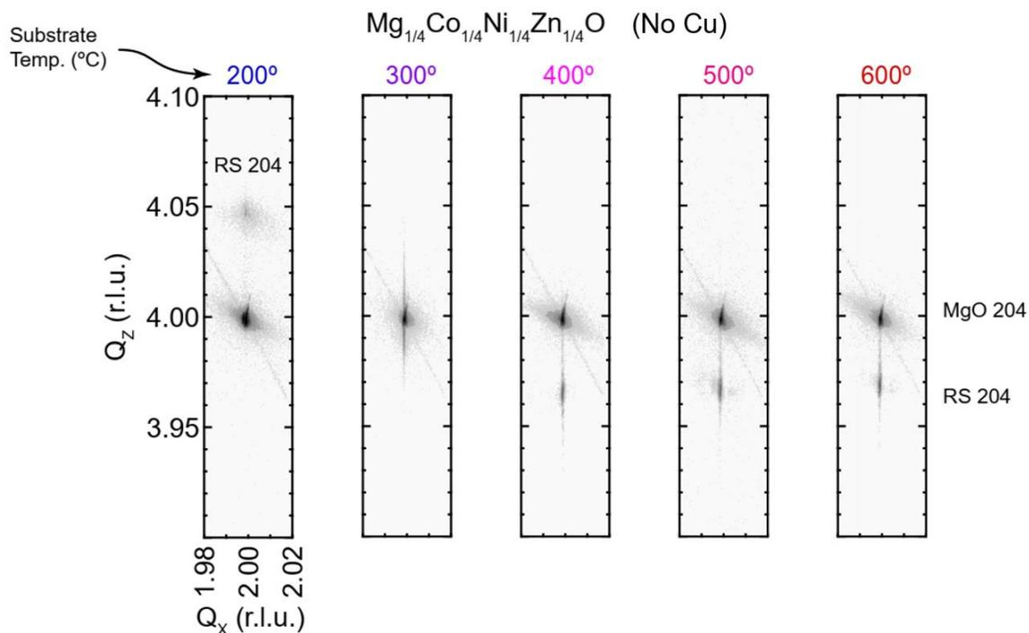
**Figure S9.** Reciprocal space maps of  $\text{Mg}_{1/4}\text{Co}_{1/4}\text{Ni}_{1/4}\text{Zn}_{1/4}\text{O}$  (No Cu) and MgO 204 reflections, indicating commensurate film growth. Substrate temperature during film growth is indicated near each plot.
