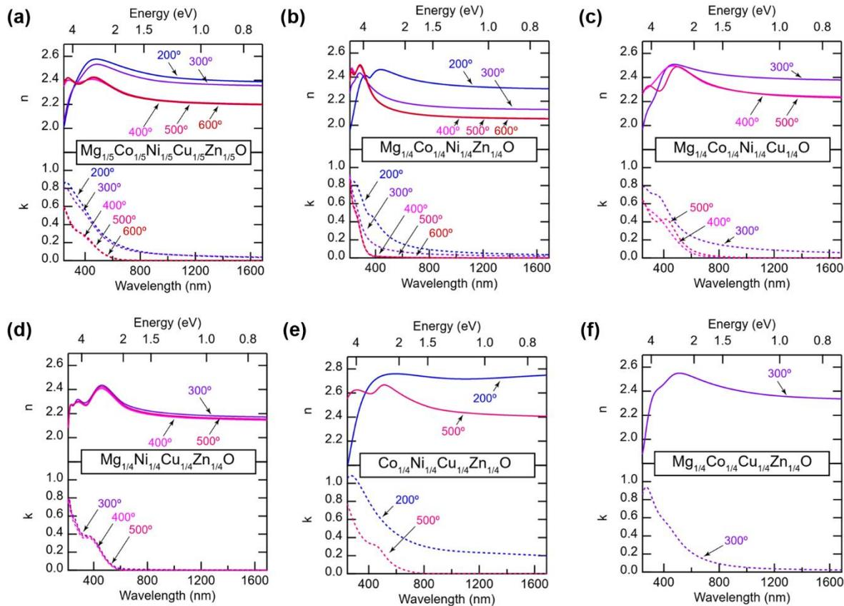
**Figure 7.** Complex refractive index models for  $\text{Mg}_{1/5}\text{Co}_{1/5}\text{Ni}_{1/5}\text{Cu}_{1/5}\text{Zn}_{1/5}\text{O}$  and four-component derivative thin films, all with the same thickness. Substrate temperature during thin film growth is indicated near each trace. Note the trend of increasing  $n$  and  $k$  with growth at lower temperatures for each composition except  $\text{Mg}_{1/4}\text{Ni}_{1/4}\text{Cu}_{1/4}\text{Zn}_{1/4}\text{O}$  (no Co).
