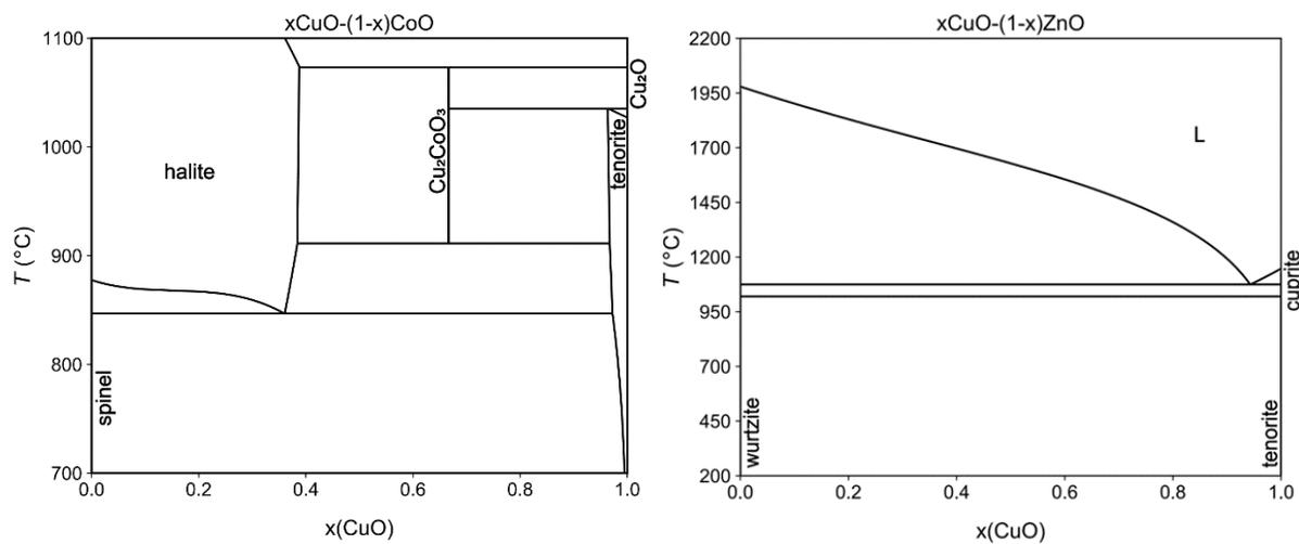
**Figure S6.** Binary phase diagrams for CuO with  $\text{Co}_x\text{O}_y$  and ZnO.
