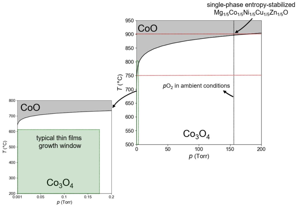
**Figure S1.** Co-O system showing CoO-Co<sub>3</sub>O<sub>4</sub> stability with temperature and oxygen partial pressure.
