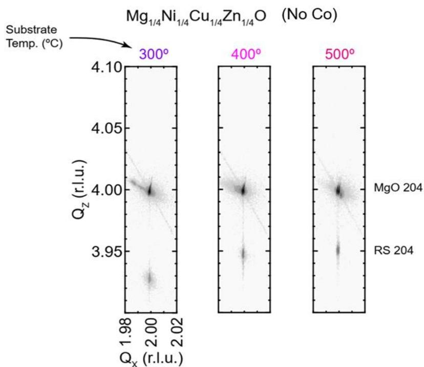
**Figure S10.** Reciprocal space maps of  $\text{Mg}_{1/4}\text{Ni}_{1/4}\text{Zn}_{1/4}\text{Cu}_{1/4}\text{O}$  (No Co) and MgO 204 reflections, indicating commensurate film growth. Substrate temperature during film growth is indicated near each plot.
