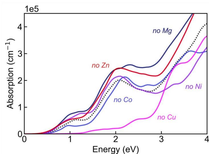
**Figure S13.** Optical absorption of parent  $\text{Mg}_{1/5}\text{Co}_{1/5}\text{Ni}_{1/5}\text{Cu}_{1/5}\text{Zn}_{1/5}\text{O}$  and its four-component derivatives.  $\text{Mg}_{1/5}\text{Co}_{1/5}\text{Ni}_{1/5}\text{Cu}_{1/5}\text{Zn}_{1/5}\text{O}$  is shown as a black dotted line.
