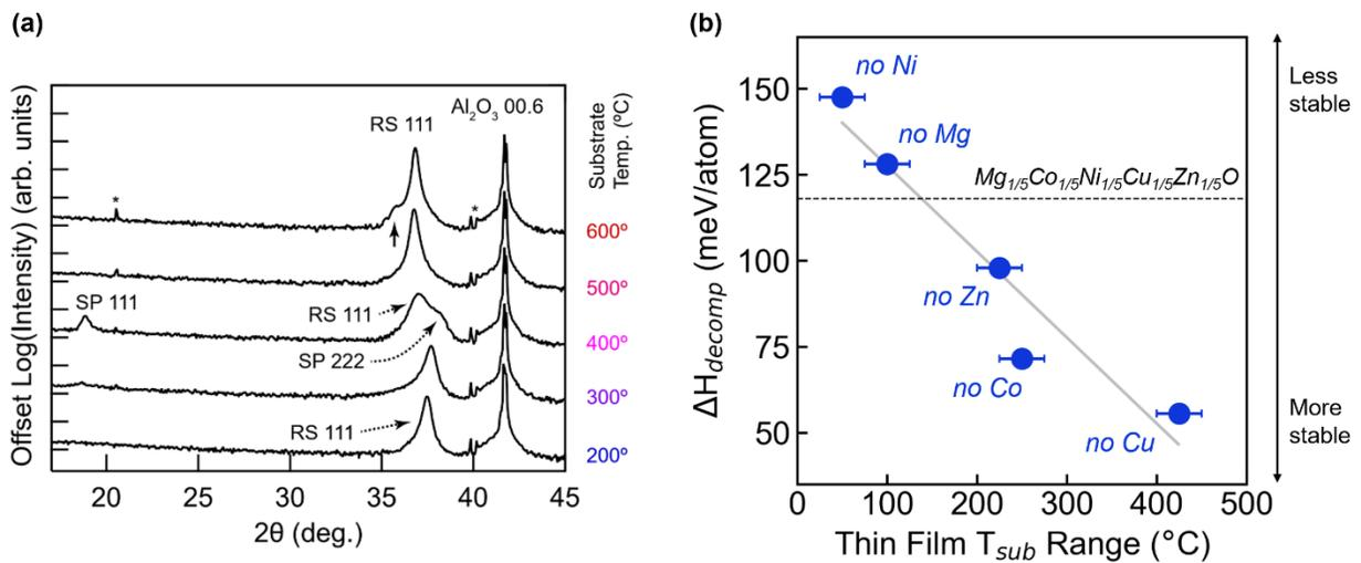
**Figure 5.** (a) X-ray diffraction patterns of  $\text{Co}_{1/4}\text{Ni}_{1/4}\text{Cu}_{1/4}\text{Zn}_{1/4}\text{O}$  (no Mg) films on [00.1]- $\text{Al}_2\text{O}_3$  as a function of temperature, (b) Single-phase substrate temperature range for rock salt thin films plotted against the DFT calculated decomposition enthalpy. Linear fit is shown as a grey line, while the five-component parent decomposition enthalpy is plotted as a black dashed line.
