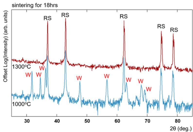
**Figure S7.** X-ray diffraction patterns of two bulk ceramics mixed from MgO, NiO, and ZnO to form stoichiometric  $\text{Mg}_{1/3}\text{Ni}_{1/3}\text{Zn}_{1/3}\text{O}$  and are sintered at 1000 °C (bottom) and at 1300 °C (top) for 18 hours. Intermediate temperatures are not shown for clarity. The wurtzite phase signatures start disappearing around 1300 °C.
