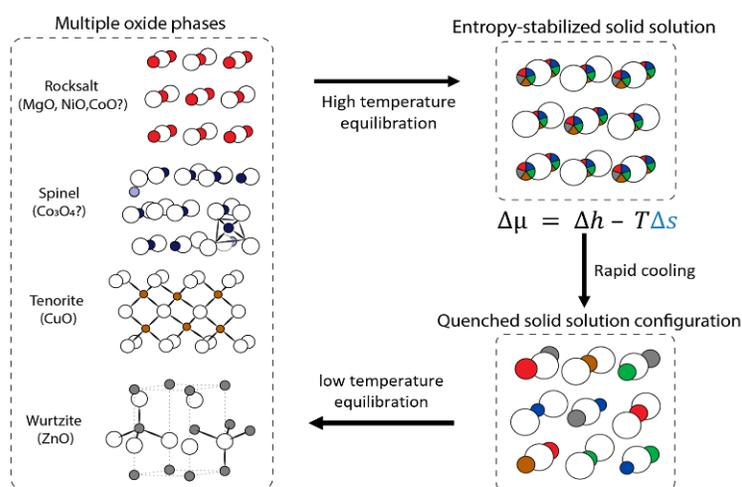
**Figure 1.** Flowchart illustrating phase progression in the  $\text{Mg}_{1/5}\text{Co}_{1/5}\text{Ni}_{1/5}\text{Cu}_{1/5}\text{Zn}_{1/5}\text{O}$  system with temperature - reproduced from our JAcers feature article [2]. We highlight in this work that in addition to  $\text{CuO}$  and  $\text{ZnO}$ ,  $\text{Co}_3\text{O}_4$  should be explicitly considered in low temperature processes.
