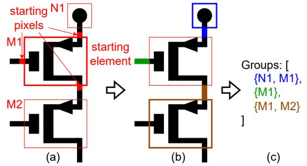
Fig. 2. Grouping neighboring components for net detection
