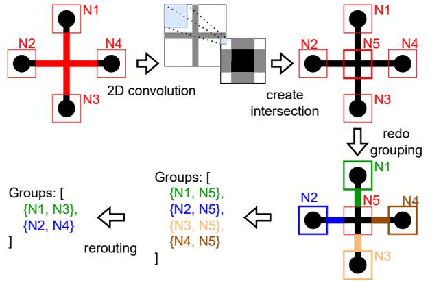
Fig. 3. Handling intersections for net detection
