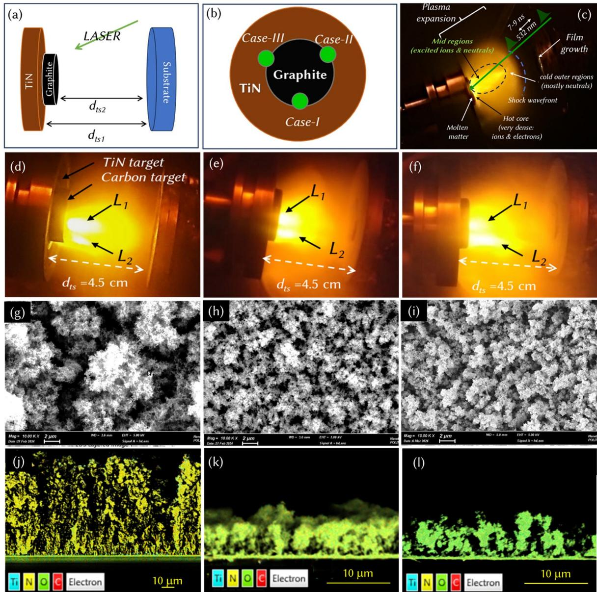
**Figure 3:** (a) Schematic of targets assembly and (b) three ablation spots. (c) Photographic image of plasma plume for single target ablation by 532 nm laser demarcating different zones of plasma. (d-f) Representative photographic image of plasma plume for three different ablation conditions. Corresponding (g-i) scanning electron micrographs, (j-l) elemental layered image.
