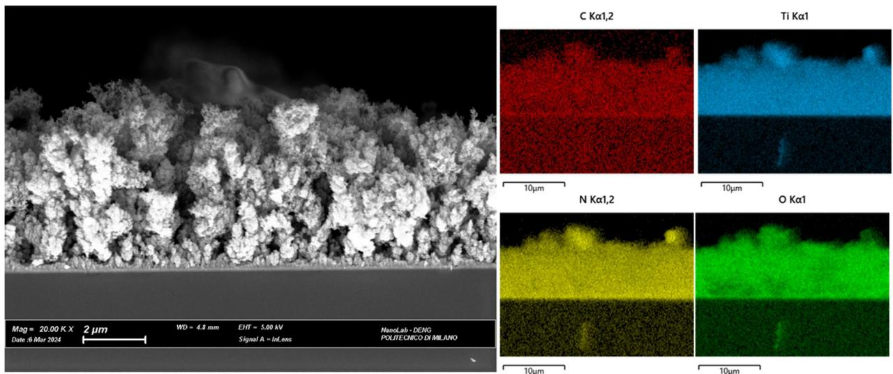
Figure S3: Cross-sectional scanning electron micrograph and elemental mapping of  $C-TiO_xN_y-3$
