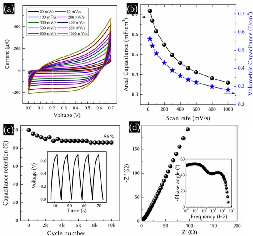
**Figure 2: Supercapacitor performance of Carbon-Titanium oxynitride.** (a) cyclic voltammogram at different scan rates, (b) areal and volumetric capacitance with respect to the scan rate, (c) cycle stability with the charge-discharge cycles at  $100 \mu\text{A}$  in an inset, (d) Nyquist plot with Bode plot in the inset.
