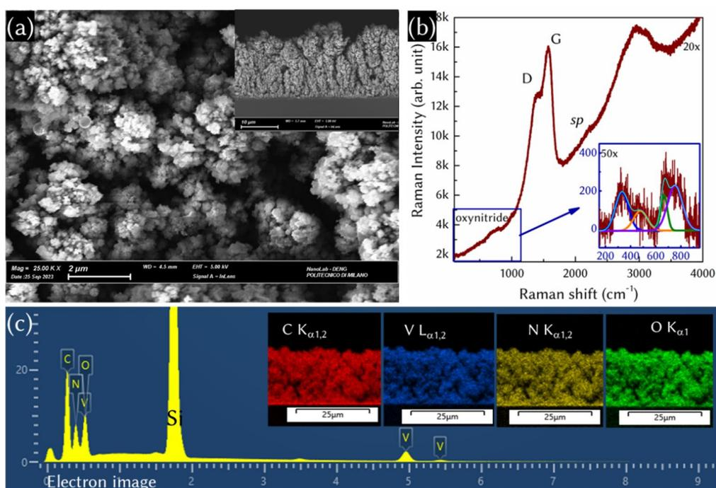
Figure 6: **Morphology and structure of Carbon-vanadium oxynitride.** (a) Scanning electron micrograph, (b) Raman spectra of nanofoam composite with low-frequency range spectra accumulated for higher time at inset. (c) EDX spectra, (d) electron image, and elemental mapping of (e) carbon, (f) vanadium, (g) nitrogen, and (h) oxygen.
