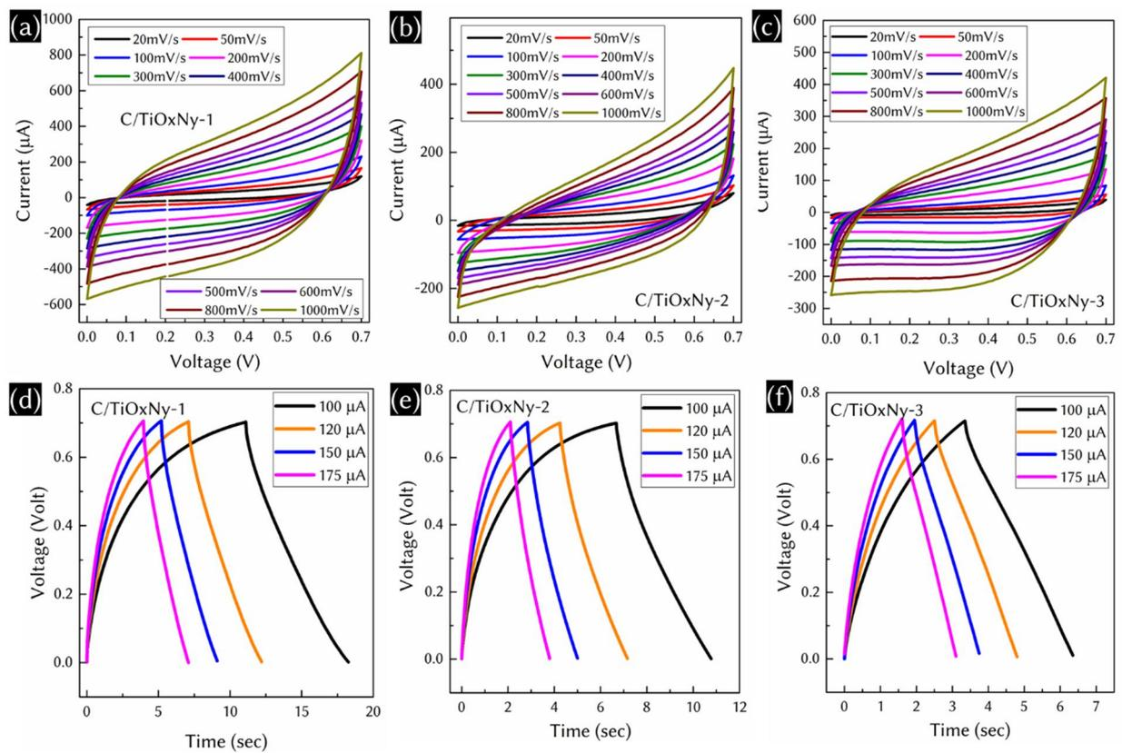
Figure S4: Cyclic voltammogram of (a)  $C/TiO_xN_y-1$ , (b)  $C/TiO_xN_y-2$ , and (c)  $C/TiO_xN_y-3$  supercapacitor device at different scan rates. Charge-discharge profile of (a)  $C/TiO_xN_y-1$ , (b)  $C/TiO_xN_y-2$ , and (c)  $C/TiO_xN_y-3$  supercapacitor device at different current densities.
