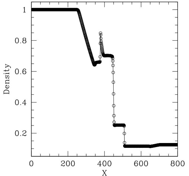
FIG. 11.— MHD Riemann problem: density vs.  $X$  at  $t = 80$  sec.
