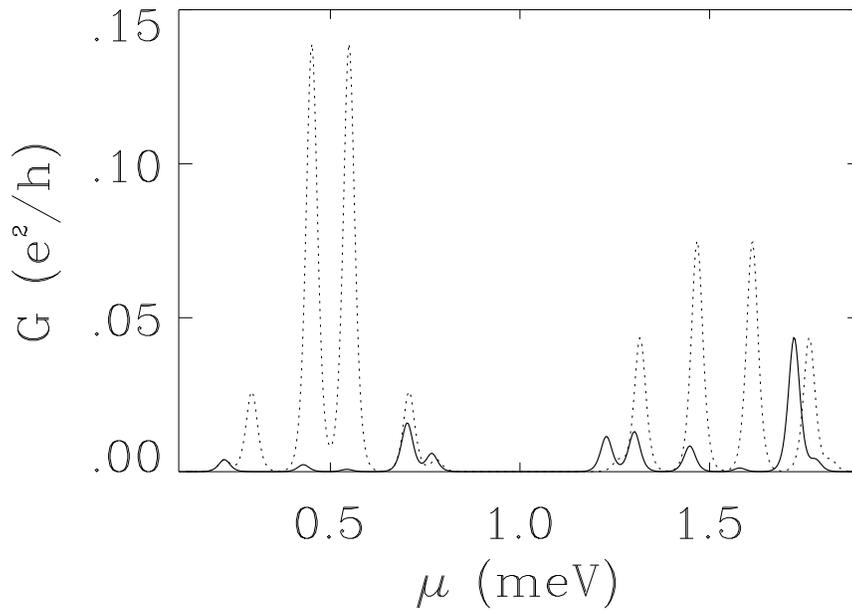
FIG. 8. Conductance vs. chemical potential  $\mu$  through a linear array of 6 GaAs quantum dots with one spin-1/2 orbital per dot.  $e^2/C_g = 1\text{meV}$ ,  $C/C_g = 0.5$ ,  $\bar{t} = .05\text{meV}$ ,  $T = 120\text{mK}$ . Spin-dependent disorder  $\delta t/\bar{t} \sim 1$  ( $t_{i\uparrow} \neq t_{i\downarrow}$ ) is included in the hopping matrix elements. Solid curve:  $B = 0$ ; dotted curve:  $B = 1.3\text{T}$ . At  $1.3\text{T}$ , the 2nd conductance peak is enhanced by a factor of 1600.
