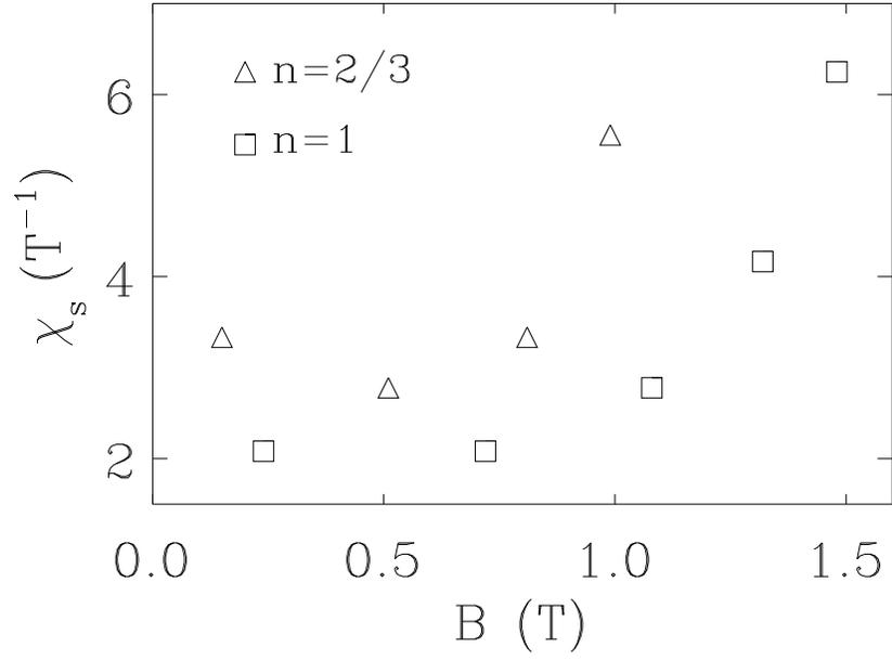
FIG. 2. Spin susceptibility  $\chi_s = \hbar^{-1}\Delta S/\Delta B$  at  $T = 0$  vs. magnetic field  $B$  for linear arrays of GaAs quantum dots with  $e^2/C_g = 1\text{meV}$ ,  $C/C_g = 0.5$ , and  $t = .05\text{meV}$ . Squares: 10 electrons on 10 dots ( $B_c \approx 1.5\text{T}$ ); triangles: 8 electrons on 12 dots ( $B_c \approx 1\text{T}$ ).
