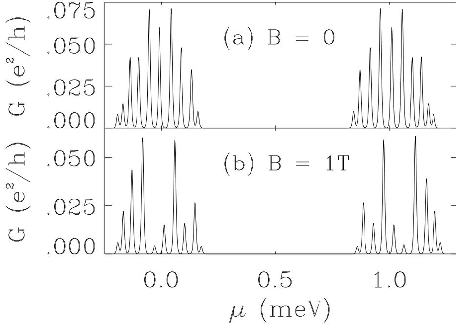
FIG. 6. Conductance vs. chemical potential  $\mu$  through a linear array of 10 GaAs quantum dots with one spin-1/2 orbital per dot.  $e^2/C_g = 1\text{meV}$ ,  $C = 0$ ,  $t = 0.1\text{meV}$ , and  $T = 35\text{mK}$ . Splitting of the two Coulomb blockade peaks into minibands is driven by  $t$ . The suppression of the 5th peak in (b) is the result of a density-dependent SPT.
