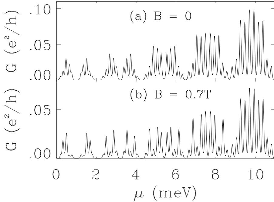
FIG. 9. Conductance vs. chemical potential through a linear array of 5 GaAs quantum dots with 5 spin-1/2 orbitals per dot.  $e^2/C_g = 1$  meV,  $\Delta = 0.2$  meV,  $T = .29$ K,  $C^{(n)}/C_g = 2^{n-1}$ , and  $t_n = 0.05$  meV $(1.05)^n$  ( $n = 0, \dots, 4$ ). The energy gap between Hubbard minibands is not resolved for  $\mu > 9$  meV (breakdown of CCB). Note the quenching of magnetoconductance effects in the ballistic regime.
