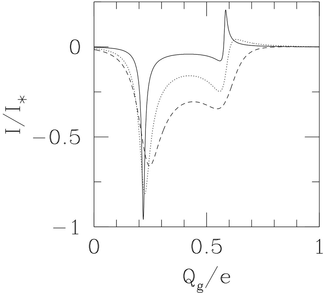
FIG. 5. Persistent current through a double quantum dot embedded in an Aharonov-Bohm ring as a function of the gate voltage. Here  $t = 1$ ,  $U = 10$ ,  $U_{12} = 0$ , and  $V_{k1} = V_{kN_d} = V$ . The current is expressed in units of  $I_* = eV/2^{1/2}\hbar$ , the value on resonance in the absence of correlations and asymmetry. Solid curve:  $V = 1/32$ ; dotted curve:  $V = 1/8$ ; dashed curve:  $V = 1/2$ .
