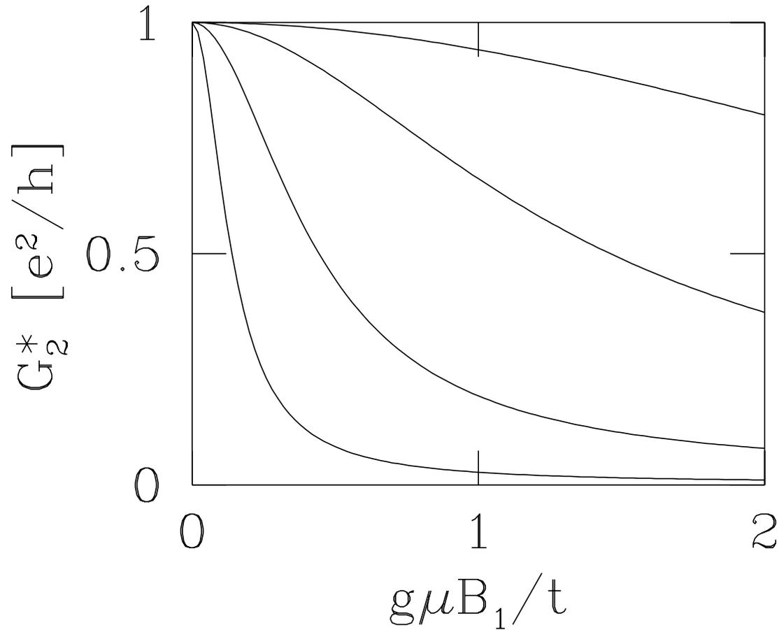
FIG. 4. Resonant conductance at  $T = 0$  in units of  $(e^2/h)/(1 + \Gamma^{(i)}/\Gamma)$  as a function of the Zeeman splitting on dot 1 for  $\gamma^{-1} = 0, 3, 10, 30$  (top to bottom). If an additional uniform external field  $B > J$  is applied, the conductance is restored to the value for  $\gamma^{-1} = 0$ , leading to giant magnetoresistance.
