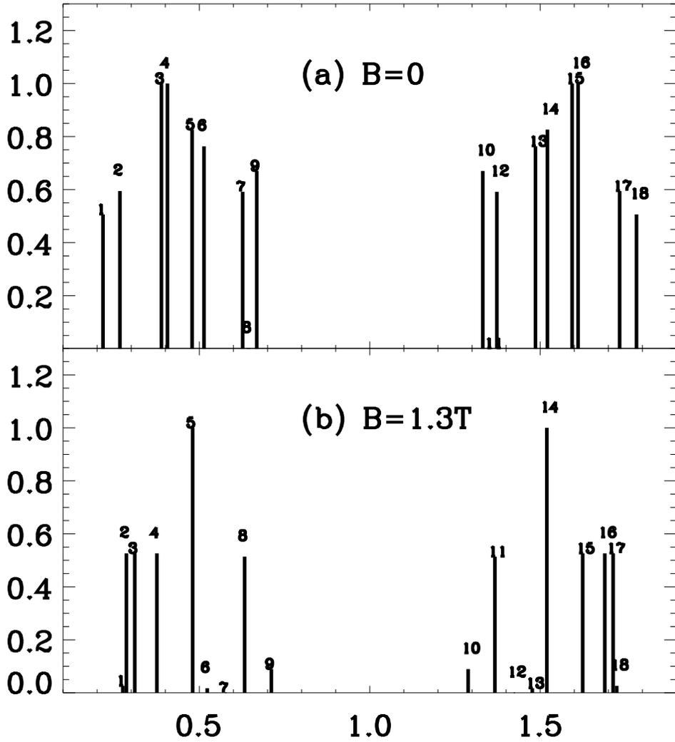
FIG. 11. The partial width  $\Gamma_N^L = \Gamma \sum_{\sigma} |\langle 0_N | d_{1\sigma}^{\dagger} | 0_{N-1} \rangle|^2$  as a function of  $N$  for the  $3 \times 3$  array of quantum dots with pure Hubbard interactions  $U = 10t$ . The widths are plotted normalized by the partial width  $\Gamma_4^L$  in (a) and  $\Gamma_5^L$  in (b). The  $x$  coordinate of the  $N$ th peak is given by  $E_N^0 - E_{N-1}^0$ . Each peak is labeled by  $N$ . The peak structure is discussed in the text.
