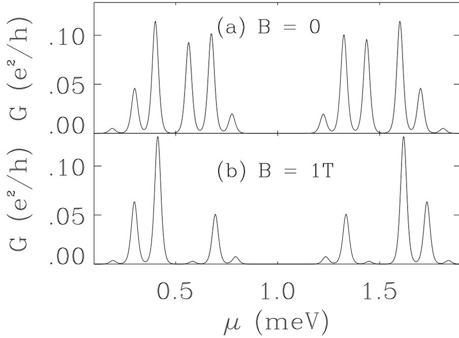
FIG. 7. Conductance vs. chemical potential  $\mu$  through a linear array of 6 GaAs quantum dots with one spin-1/2 orbital per dot.  $e^2/C_g = 1\text{meV}$ ,  $C/C_g = 0.5$ ,  $\bar{t} = .05\text{meV}$ ,  $T = 120\text{mK}$ . Disorder  $\delta t/\bar{t} \sim 1$  ( $t_{i\uparrow} = t_{i\downarrow}$ ) is present in the hopping matrix elements. The splitting of the Coulomb blockade peaks into multiplets is dominated by  $C$ ; however, the effect of  $B$  is similar to that in Fig. 1.
