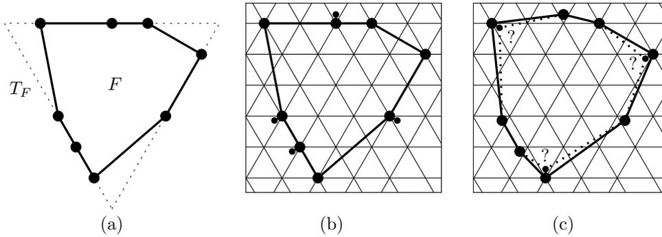
Figure 4: (a) A typical face  $F$  constructed by the convex embedding algorithm. (b) The new positions of the vertices of  $F$  which are pushed out are indicated. (c) The result of the rough perturbation. The perturbation of the vertices with question marks depends on the other faces incident to these vertices.
